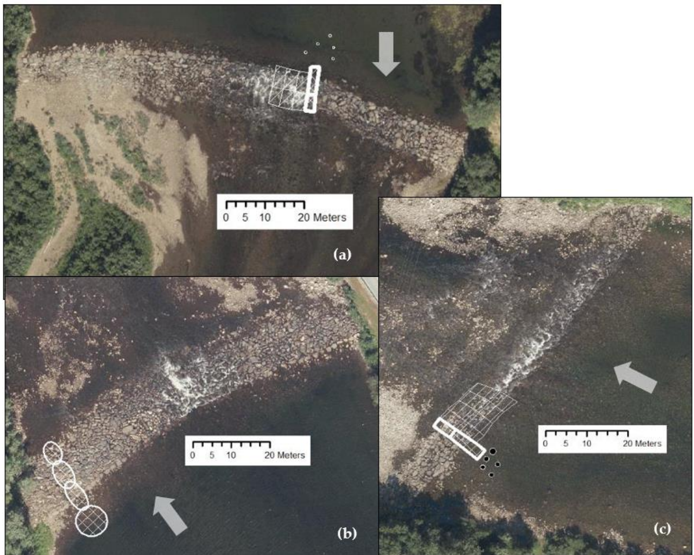
Figure 4. Polygons for weir adjustment in weirs no. 1 (a), 22 (b), and 7 (c). For (a,c), the cross-hatched, thickly outlined polygons represent a 2 m deep and wide channel across the weir, while the thin-lined polygons represent a minor lowering of the weir level, gradually increasing towards the deep channel. White-outlined black dots indicate the placement of rocks for hydraulic disruption at the entry point to the deep channel. For weir 22 in picture (b) the cross-hatched, thickly outlined polygons represent gradually lowered cell pools. The thick white arrow indicates flow direction.
