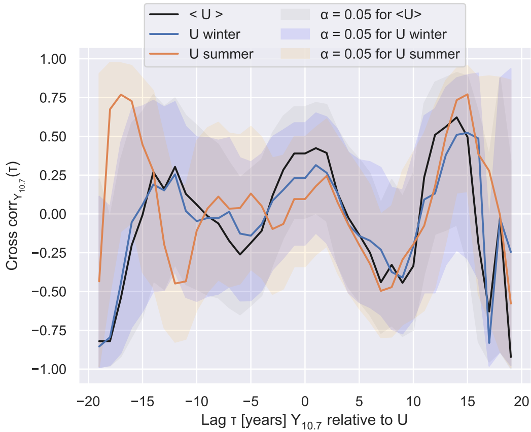
Figure 14: Cross-correlation with 95% confidence interval between yearly averages of Y_{10.7} and zonal wind averaged over full years in black, summer zonal wind in orange and winter zonal wind in blue. Negative lags refer to years the solar index leads the wind.
