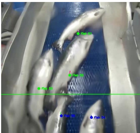
Fig. 6. Example frame showing fish being counted as they pass an imaginary line (green line). The green labels indicate that the fish has been counted, blue indicates that it is yet to be counted.
