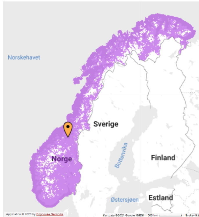
Figure 2.10: Coverage of NB-IoT in Norway by Telia. White areas are areas without coverage. Figure by Telia [41]
