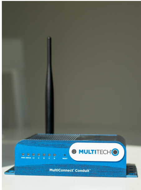
Figure 4.5: MultiTech Conduit LoRaWAN base station. Photo: Eivind Jølsgard/NTNU (CC BY 4.0)
