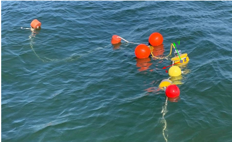
Figure 6.14: Test setup for motion verification on sea with reference frame
