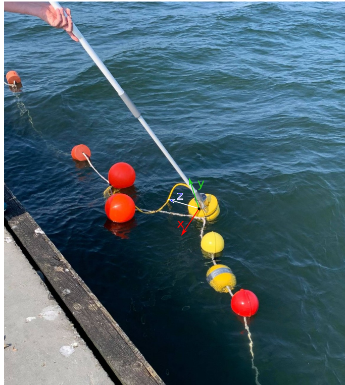
Figure 6.18: Fish movements simulated by poking the enclosure with a boat hook
