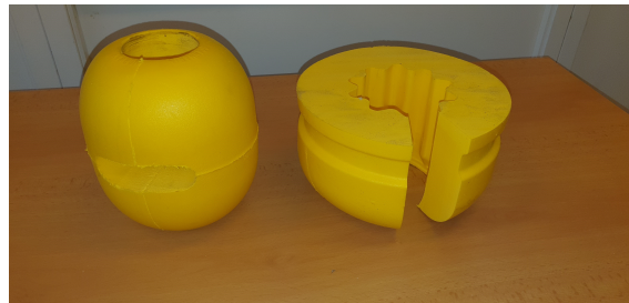
Figure 5.11: Flotation devices for load cell to the left and for enclosure on the right
