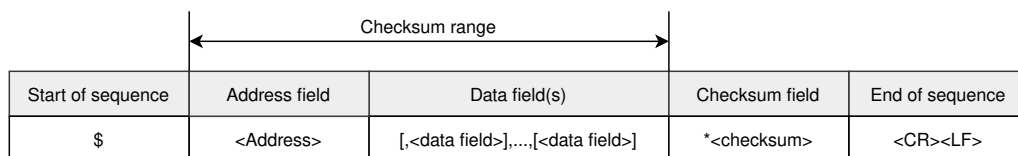
Figure 5.7: NMEA sequence structure
