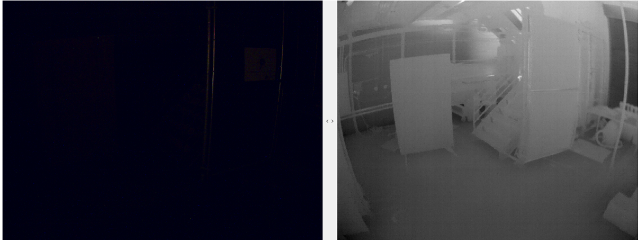
Figure 6.4: Screenshot from the lt3 sequence. It is taken after a while when the cameras are facing away from the illuminated part. Visual to the left and thermal to the right.
