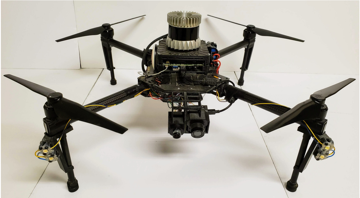
Figure 6.1: Illustration of the robot used to collect the datasets. The thermal and visual cameras are visible in the front and the LIDAR is at the top. The IMU is not visible, but below the Intel NUC. Courtesy of the autonomous robots lab.
