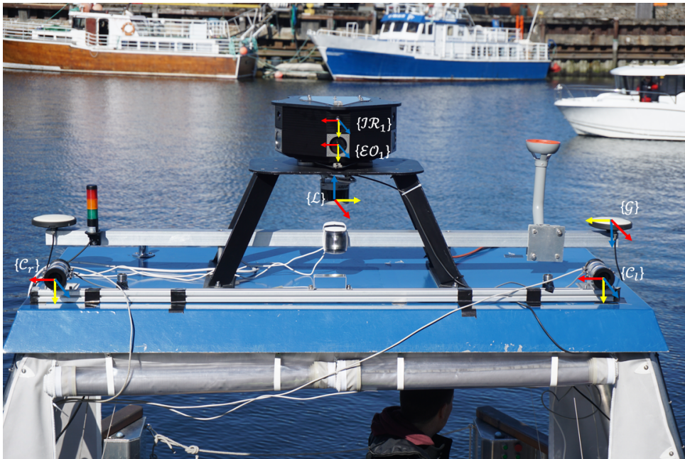
Figure 6.1.2: Illustration of the milliAmpere sensor setup listed below. Sensor frames are illustrated in the image. The red arrow depicts the x-direction, while yellow is y-direction and z is marked as blue. The sensor coordinate frames are denoted by: \mathcal{I}\mathcal{R} = infrared cameras, \mathcal{E}\mathcal{O} = electro optical cameras, \mathcal{L} = LiDAR, \mathcal{G} = GNSS, and \mathcal{C}_i = stereo cameras which is further denoted left ( l ) and right ( r ). Image captured by the author.
