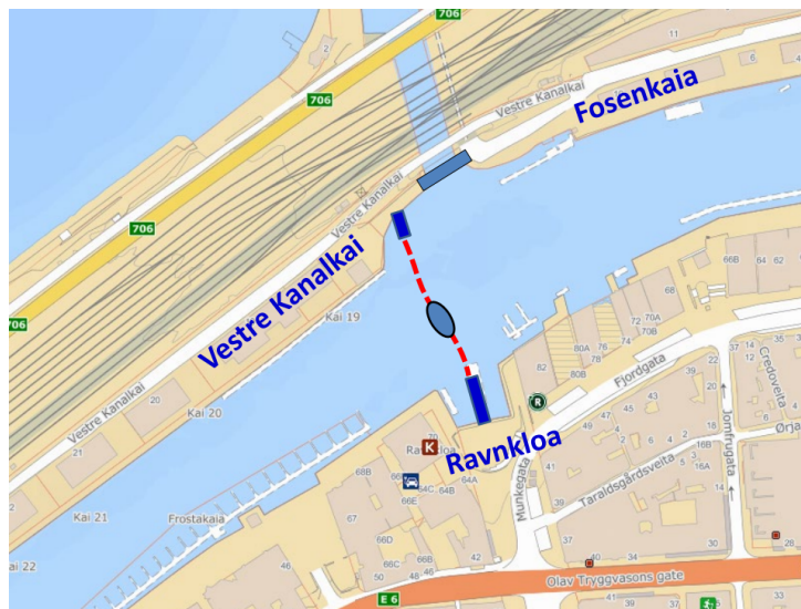
Figure 6.1.1: Intended operational region for mA2. The image shows an overview of Brattøra in Trondheim. The blue oval illustrates mA2 traveling along the striped lines, between the highlighted dark blue docking areas on Ravnkloa and Vestre Kanalkai.
