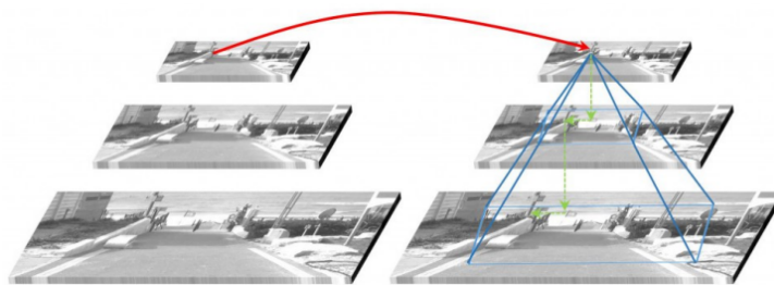
Figure 3.3.1: Image pyramid of the optical flow algorithm. The image at top of the pyramid describes the image with the lowest resolution, which estimates the initial optical flow. The estimate is refined for every level down to the original image.
