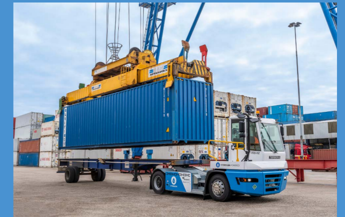
Figure 6 First concept hydrogen-powered terminal tractor [35]
