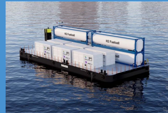
Figure 5 Example of barge providing cold ironing service with the help of fuel cells (Nedstack).
