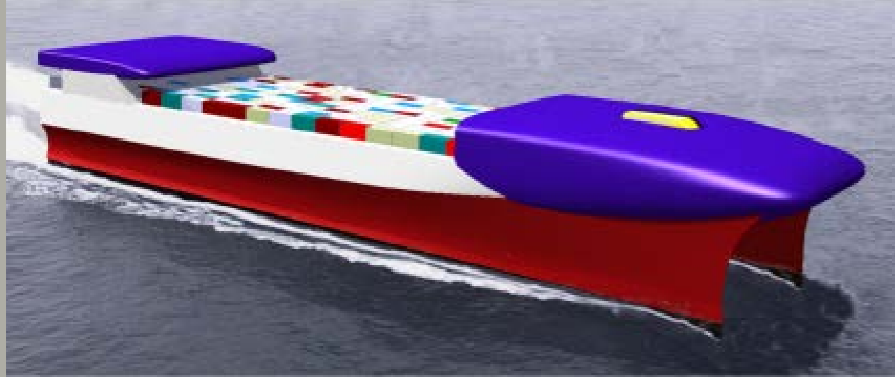
Figure 24 A hydrogen powered fast container transport designed to replace air freight [46].
