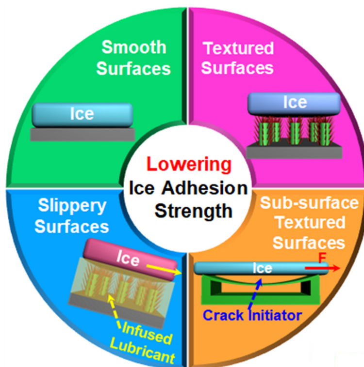
Figure 2. Strategies towards designing icephobic surfaces by lowering ice adhesion strength can be roughly divided into four types via surface properties: smooth surfaces, textured surface (i.e., hierarchical hydrophobic surfaces or SHSs), slippery surfaces, and sub-surface textured surfaces.
