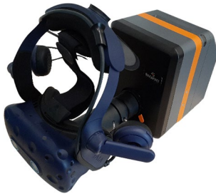
Fig. 1 HMD colorimeter calibration setup. Vive Pro Eye and I29 with AR/VR lens.
