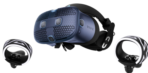
Figure 4.12: A HTC Vive Cosmos HMD and its two controllers. Taken from (Lang 2021).
