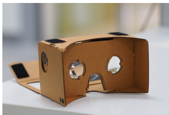
Figure 4.11: An HMD mount made out of cardboard, allowing a smartphone to be mounted inside to view VR content with some limitations. Taken from (othree 2020)
