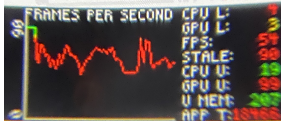
Figure 11.8: A performance graph made by the OVRMetrics tool showing the average FPS inside the Oculus Dashboard.
