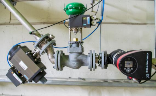
Figure 9. Hydraulic scale model control equipment (left to right: butterfly valve, globe valve, pump)
