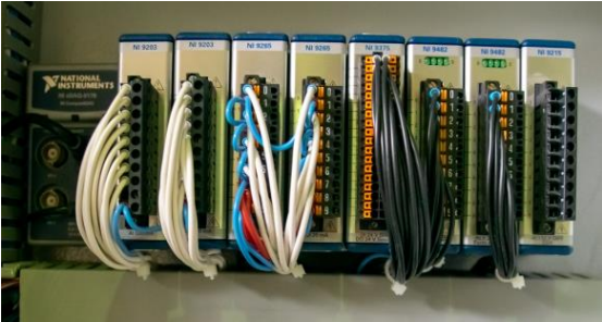
Figure 10. CompactDAQ and modules installed for hydraulic model control and monitoring
