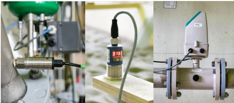
Figure 7. Measuring devices in the model (left to right: pressure sensor, ultrasonic sensor, flow meter)
