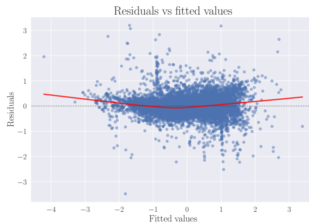
Figure 4.7: Residual plot for the linear model, where the raw residuals are plotted against the fitted values provided by the model. The red curve is a local regression line fit to the residuals to detect patterns.
