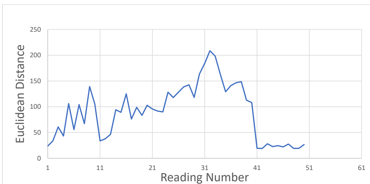
Figure 3.3 - Sensitivity trend of the sensor resulting from alteration between 30mM acetic acid and water. Plot shows variation in ED as well as sensitivity change over time, odd reading number (1,3,5,...) represent water resting while even reading numbers (2,4,6,...) represent acetic acid solution resting in sensor array container.
