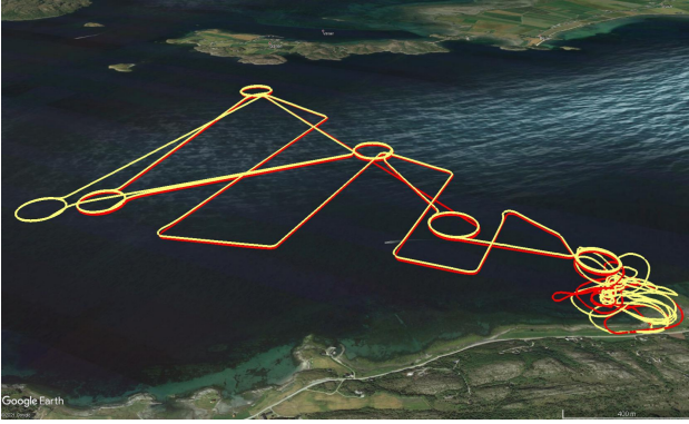
Fig. 3: Flight paths of the UAV based on RTK GNSS (yellow—flight 1, red—flight 2)
