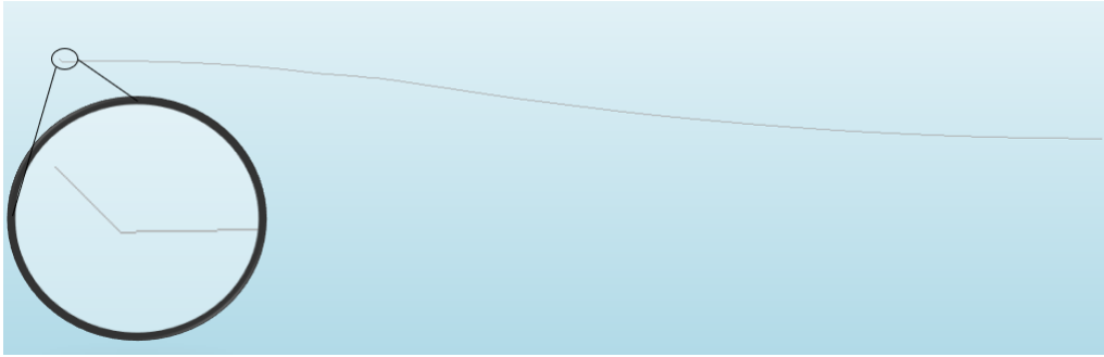
Figure 72: Tendon shape with applied parameters k_{n,w} = 0,1 and k_{t,w} = 0,001
