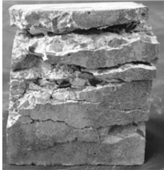
Figure 67: Yielding in biaxially loaded fatigue specimens[25]
