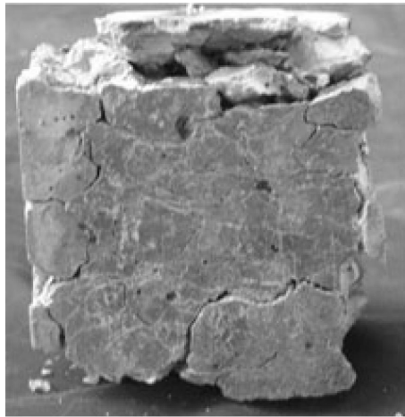
Figure 11: Failure mode of plain concrete cube due to uniaxially cyclic loading[25]
