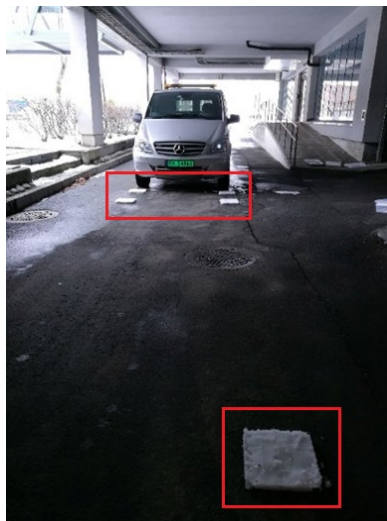
137 Figure 1. Placement of snow sample (marked in red) prior to testing.
