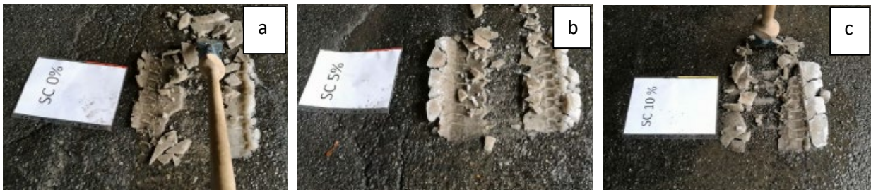
189 Figure 3. Showing snow with solution contents of 0,5 and 10 wt.% respectively after a scraping test. The snow, for 0 190 and 5 wt.% solution contents detached from the pavement in flakes, as can be seen in image 3 a) and b).
