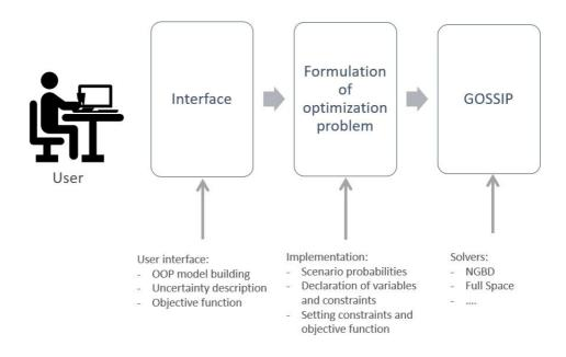
**Figure 5.1:** An overview of the different layers of code in the framework. User input is sent through the user interface to formulate an optimization problem that can be solved using GOSSIP. The internal information flow in and between *interface* and *formulation of optimization problem* is illustrated in the process flowsheet in Figure 5.2.
