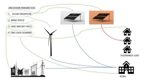
**Figure 6.5:** A simple illustration of the physical system in case study 3. The grey and red solar panels represent solar photo voltaic and thermal panels, respectively. Blue and red arrows represent electricity and heat flow, respectively.
