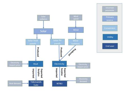
**Figure 6.6:** Flowsheet of a more complex system illustrating the different objects and relationships in the program listed on page 58. Produced, exported, surplus and imported are system variables.
