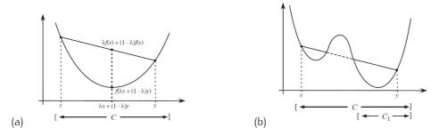
Figure 2.3: Convex (a) and nonconvex (b) function [2].
