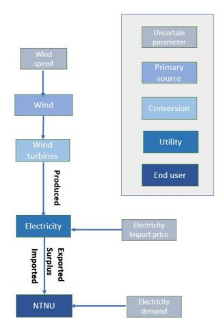
**Figure 6.2:** Flowsheet illustrating the relationship between objects in the renewable energy system illustrated in Figure 6.1. The corresponding user input model is shown in Listing 6.1. Produced, exported, surplus and imported are system variables.
