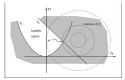
Figure 2.1: Geometrical representation of a constrained optimization problem [1].
