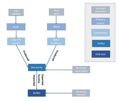
**Figure 6.4:** Flowsheet illustrating the relationship between objects in the renewable energy system illustrated in Figure 6.3. The corresponding user input model is shown in Listing 6.2. Produced, exported, surplus and imported are system variables.
