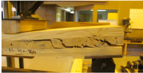
Figure 2.8: CLT: Rolling shear failure occurring in a perpendicular layer under normal bending [14]
