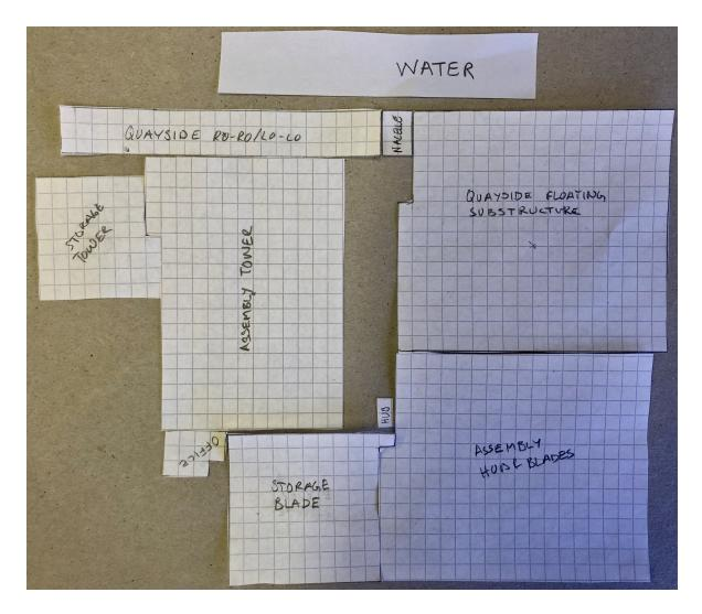
Figure 26: Port design based on Direct and Central flow of components
