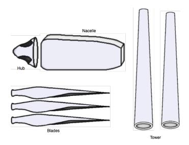
Figure 5: Turbine parts
