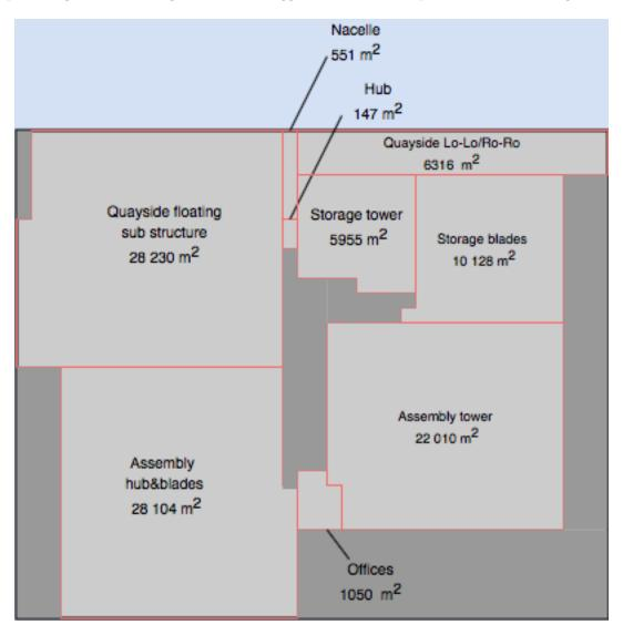
Figure 29: Final layout design: design based on relationship diagram
