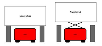
Figure 11: SPMT lifting nacelle/hub
