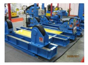
Figure 15: Pipe turning roll [37]
