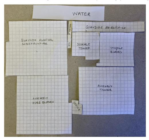
Figure 25: Port layout based on relationship diagram
