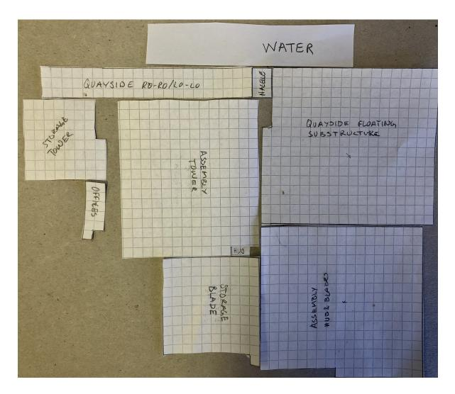
Figure 28: Port design with advantages from direct and central and relocated main aisles
