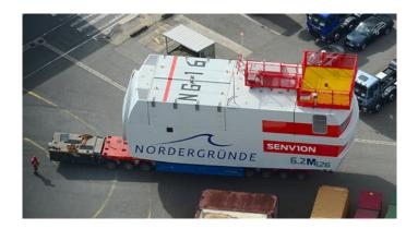
Figure 10: Nacelle on SPMT[12]
