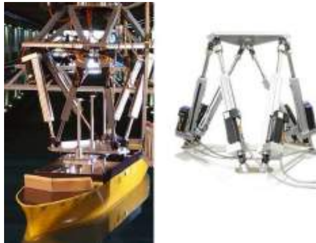
Figure 3.13: Hexapod system, Symmetrie Mistral 800 (15) (right). Vessel mounted onto the hexapod (left),
