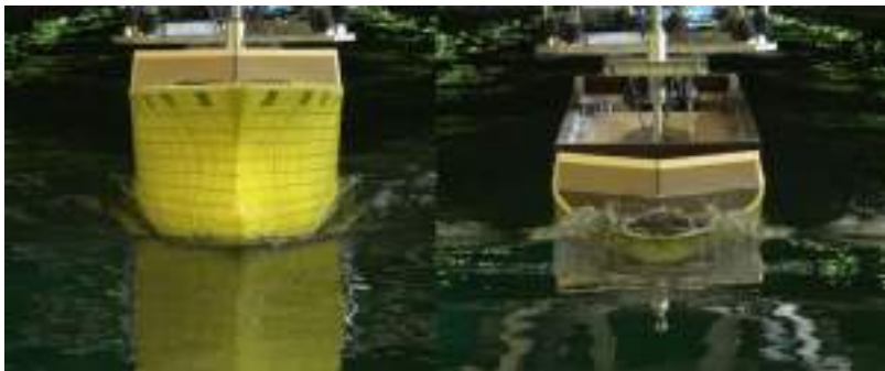
Figure 5.30: Deck slamming observed at \lambda/L = 1.4
