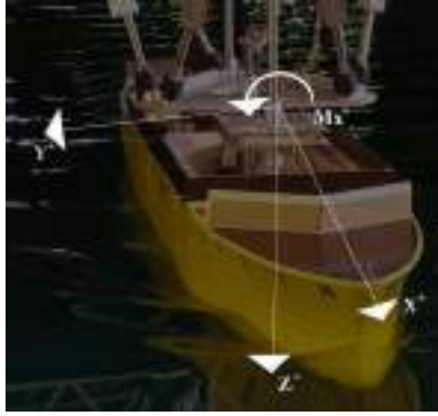
Figure 3.24: Seakeeping Cartesian coordinate system followed as per right hand thumb rule
