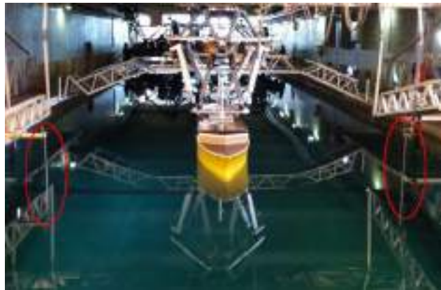
Figure 3.21: Wave probes 3 Wave probe 4 placed near model to measure incident wave elevation. It is to be noted that during following sea conditions, wave probe 3 and wave probe 4 were switched in positions after re calibration, due to lack of cable length for one of them
