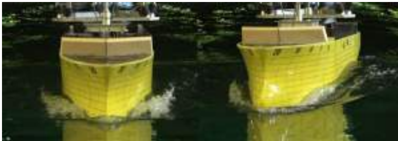
Figure 5.16: Vessel at Fn=0.179 with 0^\circ (left) and 9^\circ (right) drift angles in wavelength corresponding to \lambda/L = 1.4 . No notable separation is observed.
