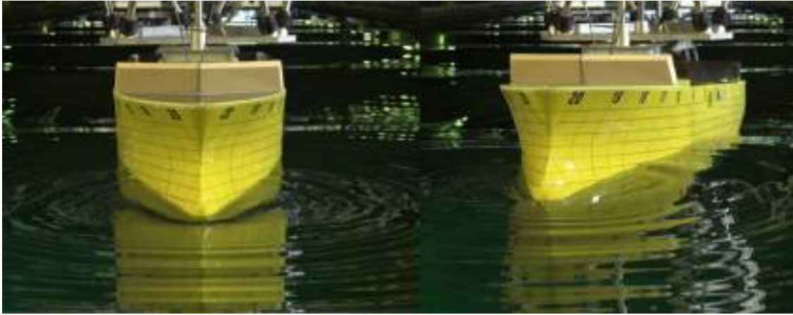
Figure 5.9: Vessel model at 0^\circ (left) and 9^\circ (right) at Fn = 0 in wave length corresponding to non dimensional wavelength \lambda/L = 1.6 . The waves generated at 0^\circ and 9^\circ are similar. No separation effects are observed in presence of a drift angle.
