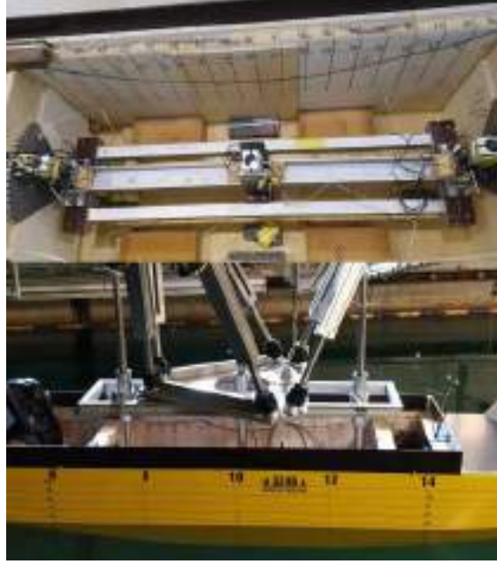
Figure 3.5: Sailboat dynamometer fixed on SOShip, The element fixed onto the model (top), Frame and rods which connects the dynamometer on the model to the carriage (bottom)
