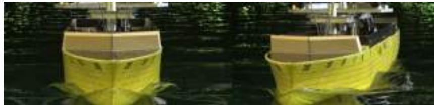
Figure 3.29: F_n=0.179 Vessel model at 0°drift angle (Left) and vessel model at 9°drift angle
