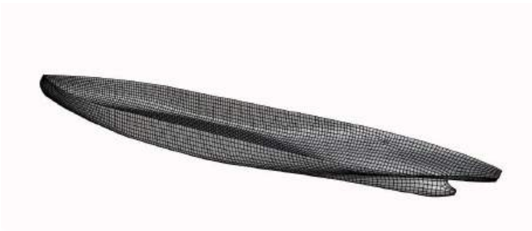
Figure 2.12: Figure illustrating the panel distribution of the wetted ship hull surface
