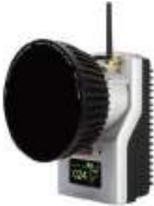
Figure 3.7: OQUS motion capture cameras by Qualis used for measuring motions along 6 DOF
