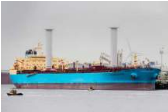
Figure 1.3: Flettner rotors installed on the Maersk Pelican 109,000 DWT tanker. (3)
