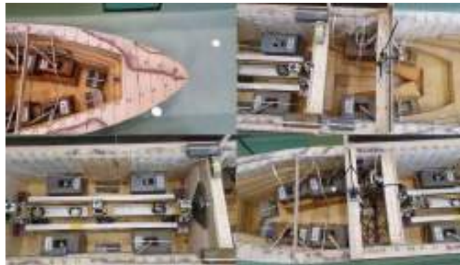
Figure 3.15: Weights placed in model to achieve the design draft ensuring an even keel
