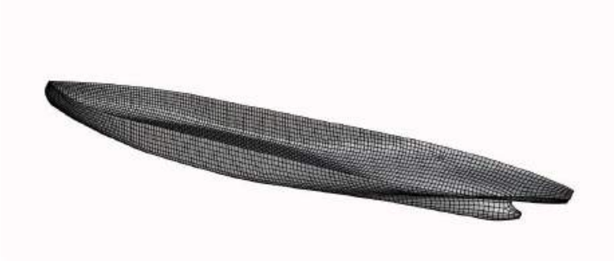
Figure 4.2: 3D panel model of SOShip used for numerical analysis
