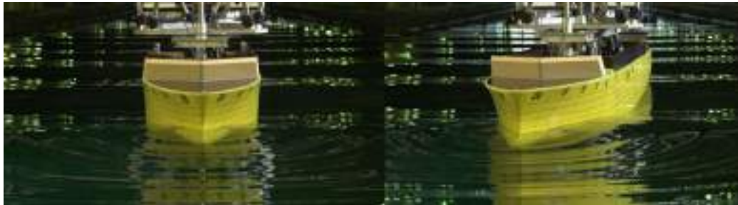
Figure 3.26: F_n=0 Vessel model at 0^\circ drift angle(Left) and vessel model at 9^\circ drift angle(Right)
