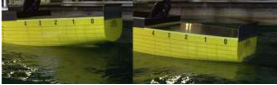
Figure 5.31: Stern slamming observed at \lambda/L = 1.4
