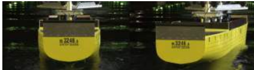
Figure 3.30: F_n=0.179 Vessel model at 180°drift angle (Left) and vessel model at 189°drift angle
