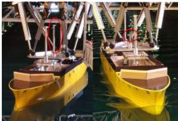
Figure 3.23: Replacing center rod (Left) from sailboat dynamo meter to frame with a rod (Right) of better vertical tolerance.
