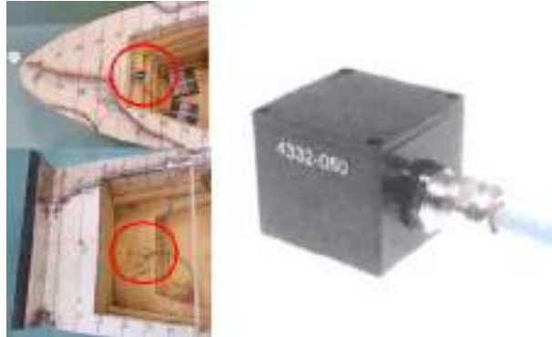
Figure 3.10: Model 4332 triaxial Accelerometer (right) used as accelerometer 16426 16316 placed in aft and fore ends(left) respectively as shown in figure 3.11
