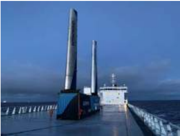
Figure 1.2: Econonwind’s ventfoil system on DFDS cargo vessel Lysbris Seaways. (3)
