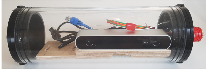
Figure 3.5: The cylindrical underwater housing containing the ZED stereo camera.
