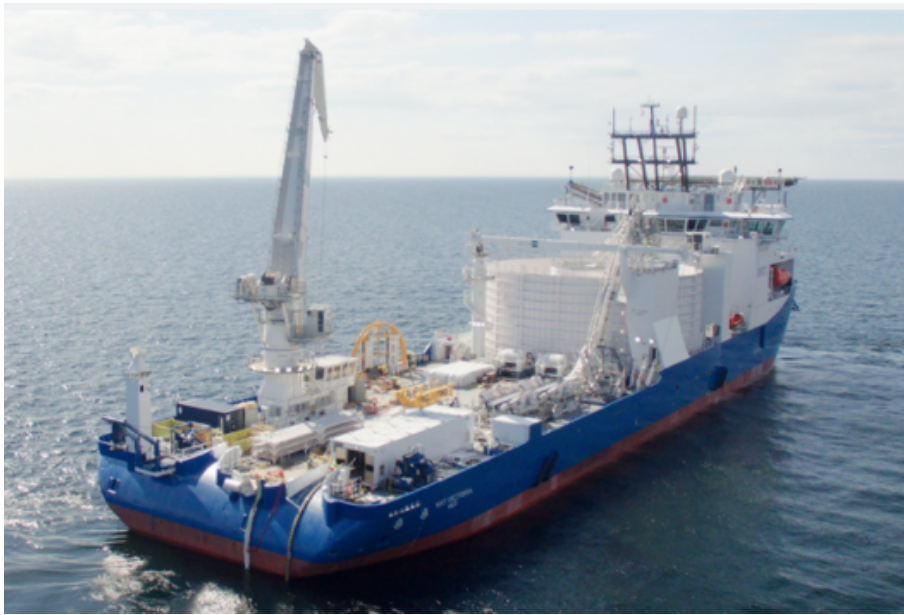
Figure 2.19: Cable laying vessel (Management, 2017)
