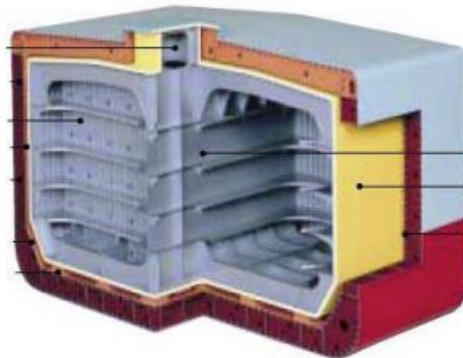
Figure 4.4: Type B tank (Boulougouris and Chrysinas (2015))
