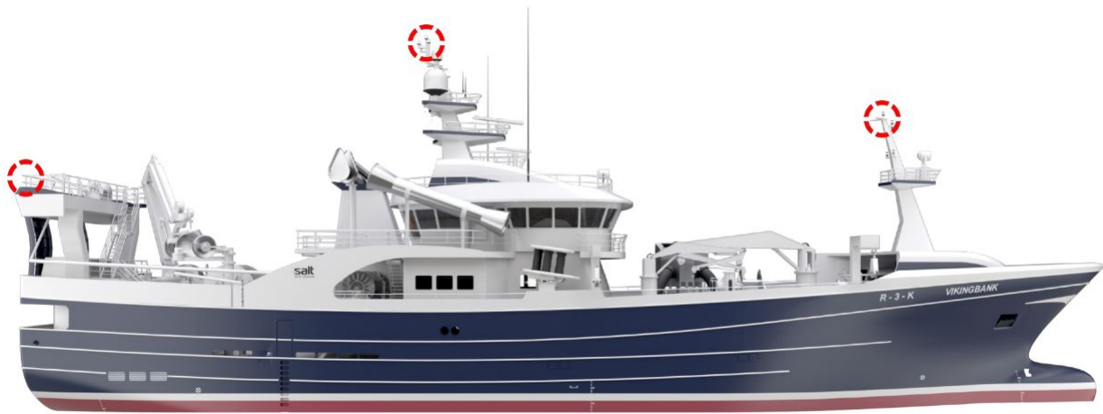
Figure 12.9: Potential placements areas of ventilation outlets
