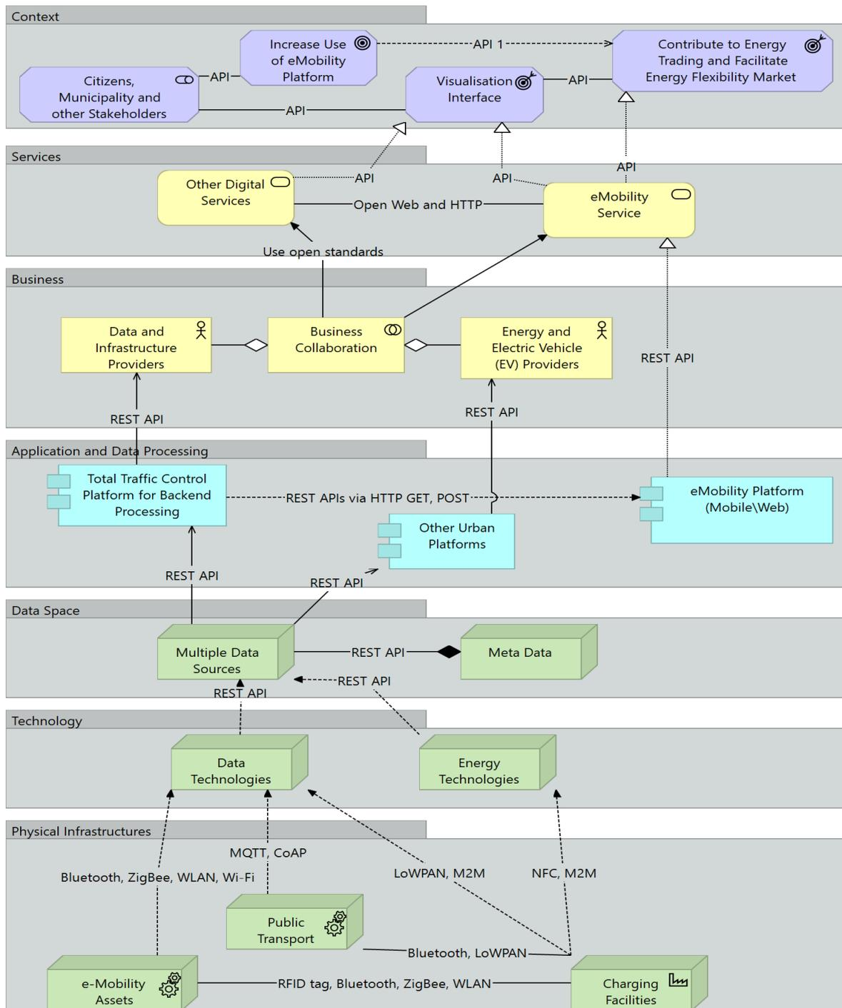
Figure 6. Meta-model to support pluggability and integration of pervasive platforms
