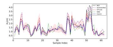
Fig. 11. Estimation of significant wave height by different approaches.
