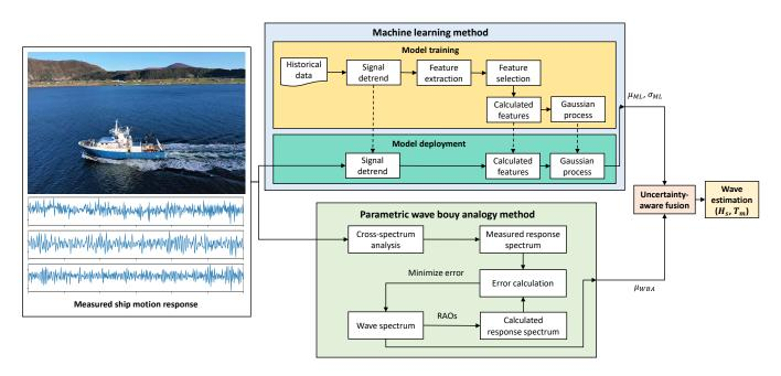
Fig. 1. Schematic illustration of the proposed hybrid approach. The upper rectangle is the ML model and the lower rectangle is the model-based method.
