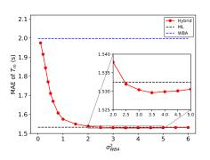
Fig. 10. Effect of  $\sigma_{WBA}^2$  on the estimation error of the mean wave period.
