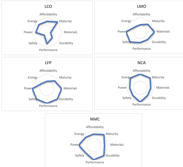
Figure 2.2: Characteristics of the most common LiB chemistries. Reprinted from Zubi et al. [16]
