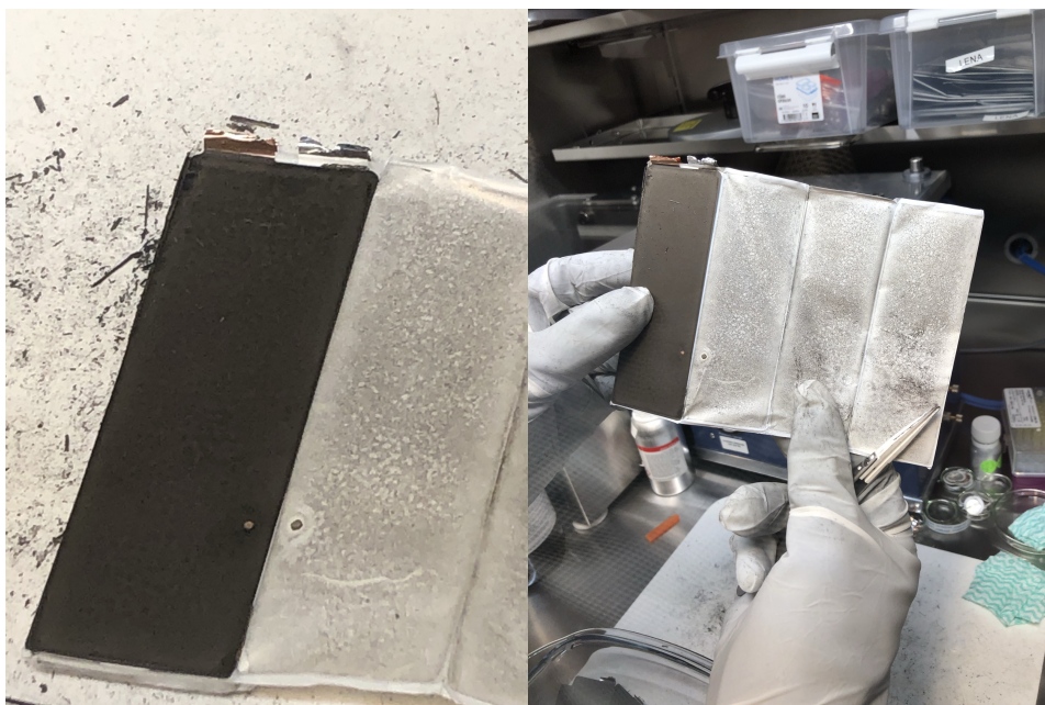
(a) Cracking of the electrode, also note the graphite dust (b) Delaminated electrode with graphite rests on the separator around the cell
