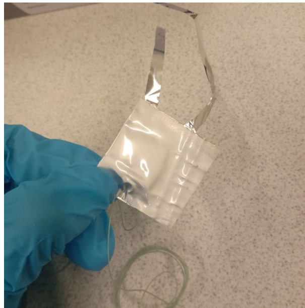
Figure 4.11: Picture of the temperature calibration cell used. The thermocouples were introduced in one side of the cell, and that side was sealed using thermal bonding film.
