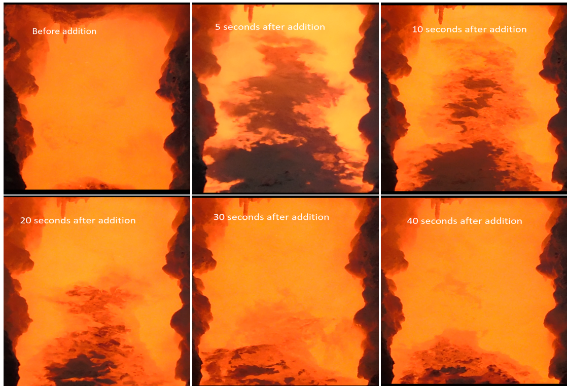
Figure 2.8: Figure showing a dissolution experiment done in an industrial cell at Alcoa Mosjøen. Experiment done by Vegard Aulie
