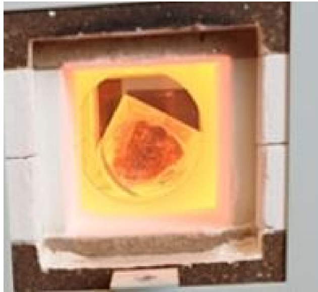
Figure 2.18: Picture of a destroyed crucible inside the see through furnace. The experiment were performed by Aulie [18] at 14.10.2019
