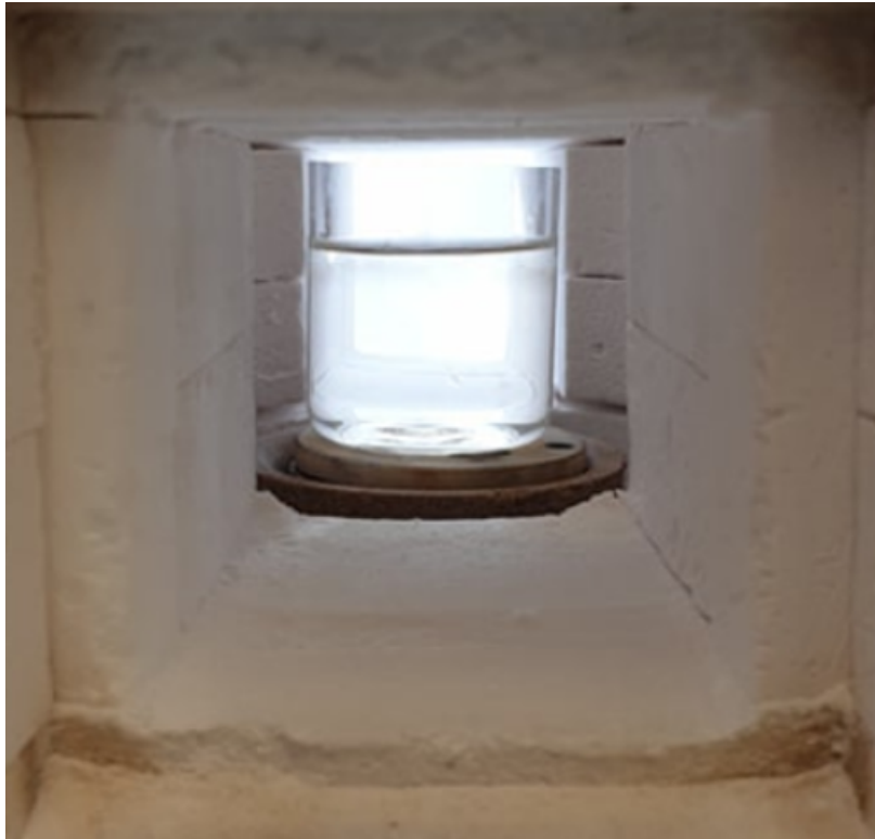
Figure 3.2: Picture of the see through cell with both shutters open and a crucible filled with water inside.
