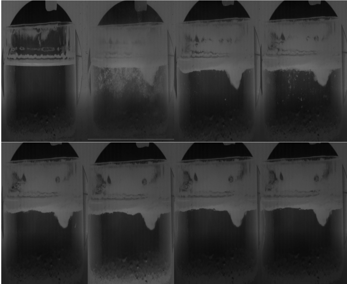
Figure 2.19: Dissolution of alumina in a see through cell. Pictures are from before addition, 5 seconds after addition, 30 seconds, 60 seconds, 120 seconds, 180 seconds, 240 seconds and 300 seconds respectively. The experiment was done on 20.11.2019 by Aulie [18].
