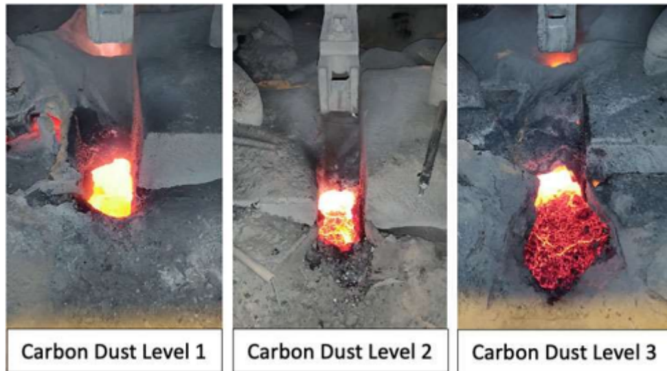
Figure 2.11: Figure showing carbon dust levels in the tap hole from [21]. Level 1 shows a tap hole with no carbon dust, level 2 shows a low amount of carbon dust while level 3 shows a high amount.
