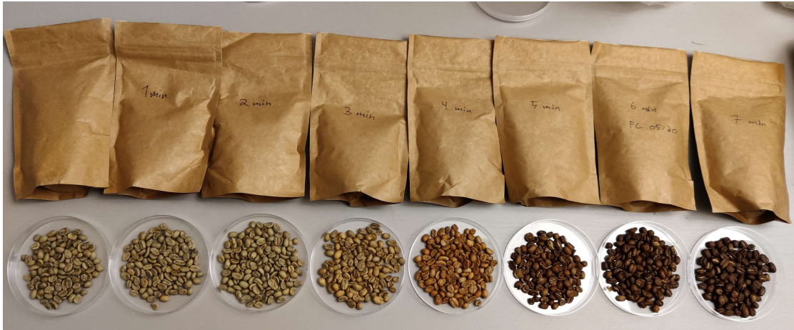
Figure 3.8: Coffee beans roasted from zero to eight minutes, left to right, using the ROEST standard roasting profile defined by table 3.1 with dropTemp = 220 and endTemp = 250
