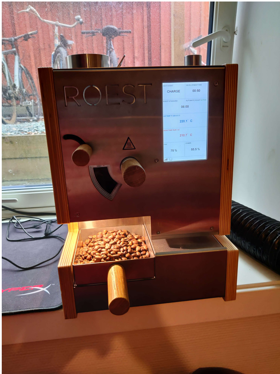
Figure 1.2: The ROEST sample roaster is a lab tool for coffee roaster made to roast 100g samples of coffee at a time.
