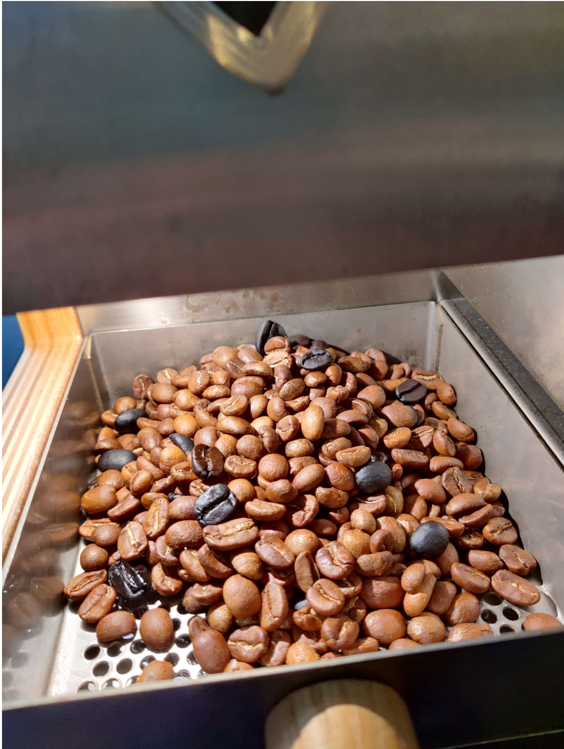
Figure 5.19: Some beans get stuck in the roasting chamber and come out much darker than the other beans in the next roast.
