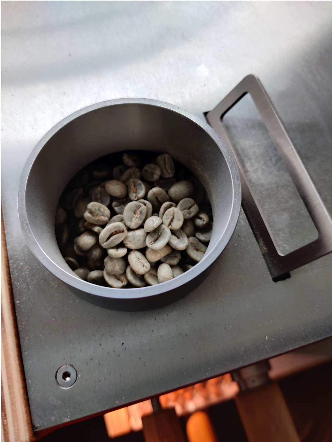
Figure 3.2: A sample is loaded in to the hatch of the ROEST sample roaster immediately before dropping into the roasting chamber.
