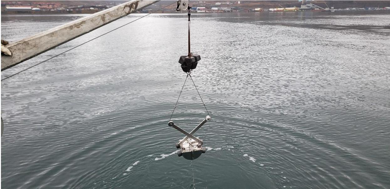
*Figure 6 Van Veen Grab in closed position connected to the crane on Polaris, the research boat used in this study*
