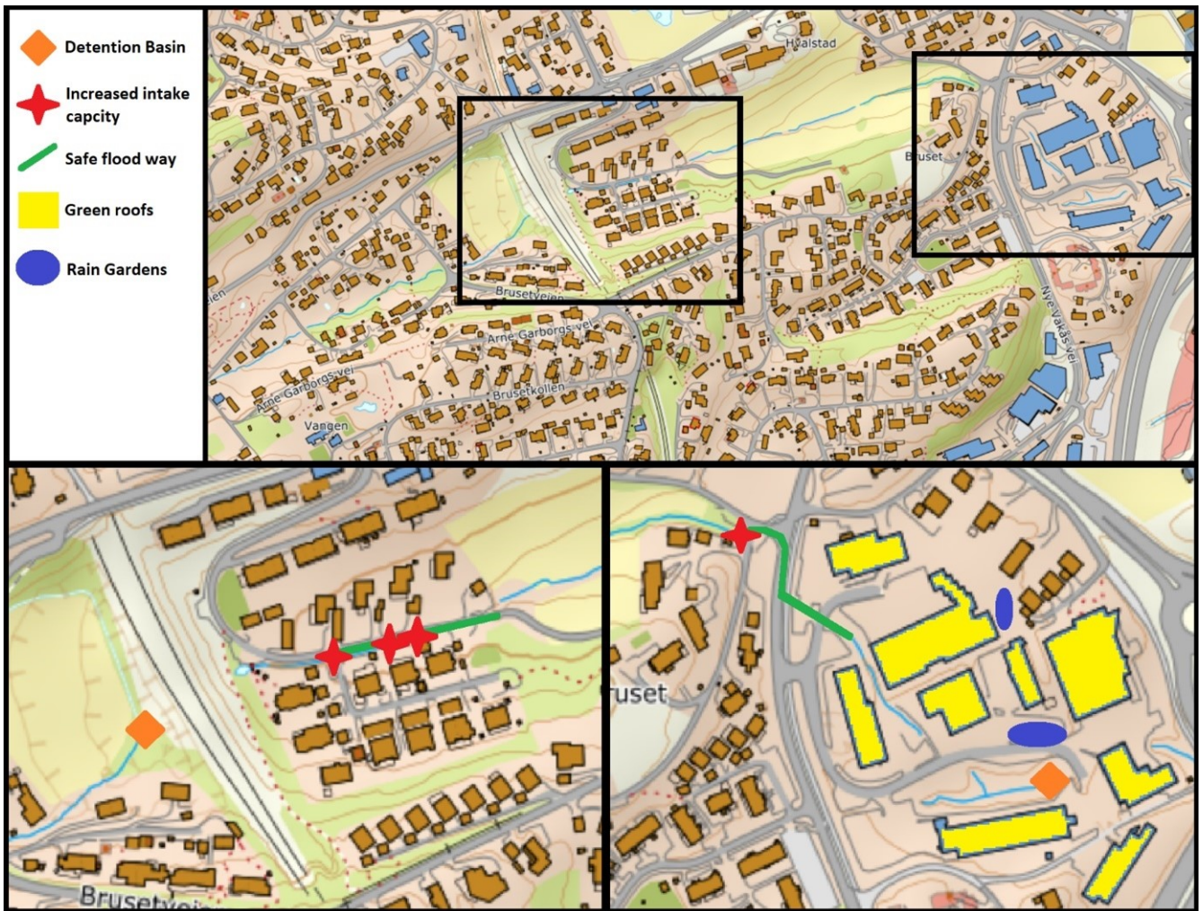
Fig. 4: Overview of stormwater control measures. Downspout disconnections not included here. For downspout disconnections, see Table 3
