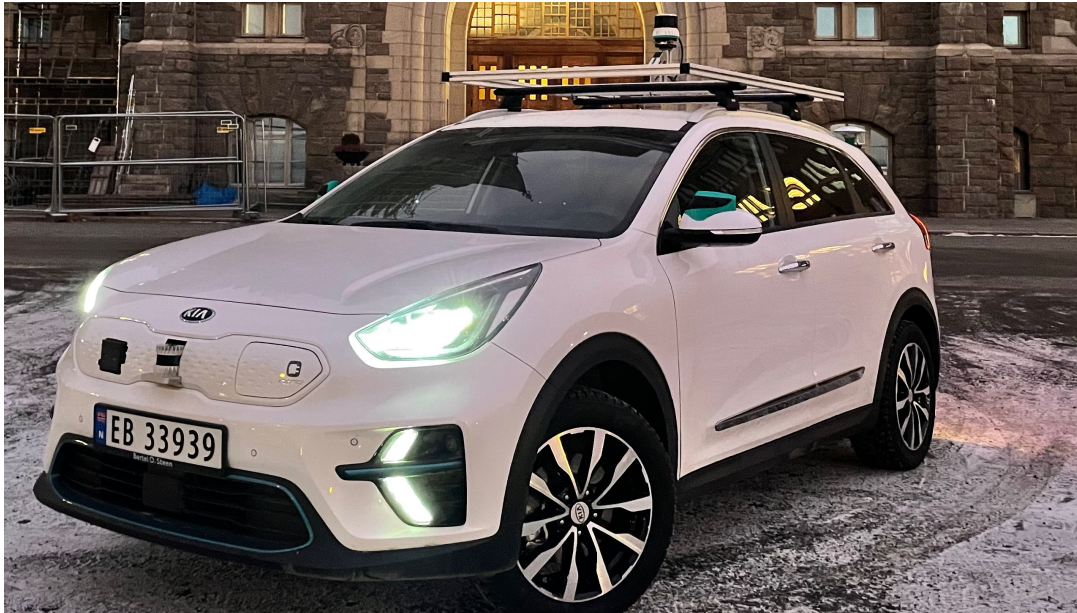
Figure 3.9: The NAP-lab Vehicle. NAP-lab’s vehicle is a Kia e-Niro equipped with sensors, a drive-by-wire-kit, and computational hardware. This equipment makes it possible to use this vehicle as a platform to develop software for autonomous vehicles
