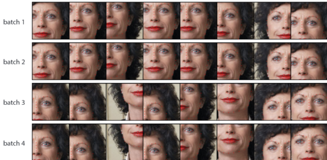
Figure 3.2: A visualization of the batch augmentation issue which commonly arises when using multiprocessing with PyTorch and NumPy. In this case, there are two workers. The first worker produces batch 1 and 3, while the second worker produces batch 2 and 4. Because the RNG states of the workers are identical, they both produce the same augmentations. The image is taken from the blog post of Tanel Pärnamaa and showcases the issue in an official PyTorch example.
