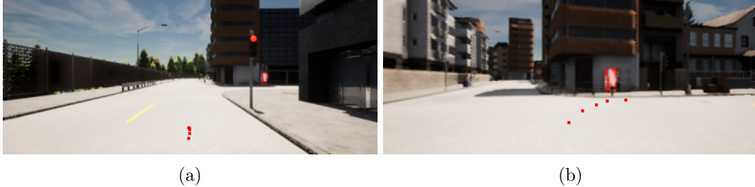
Figure 2.10: Visualization of how waypoints can be used as an output modality. The waypoints are shown as red dots. (a) Contracted waypoints, indicating full stop. (b) Arcing waypoints, indicating the path through a turn.
