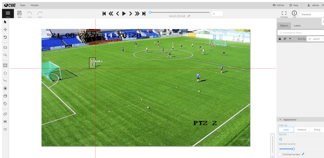
Figure 31: A snapshot of the labeling process. We used the marker to place boxes around the players and labeled each with an ID. The process is then repeated for each frame in the sequence. The same ID was used for corresponding objects between frames.
