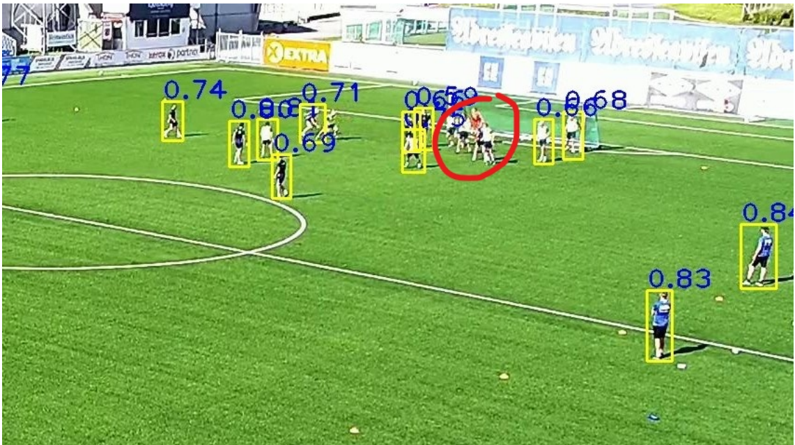
Figure 53: Examples of bad detections by the finetuned YOLOv5 model. On Ranheim validation frames, YOLOv5 frequently miss groups of players. There is a tight cluster of players in front of the goal that are not detected.
