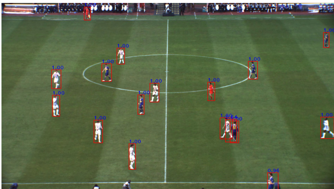
Figure 70: Examples of bad detections by the finetuned Faster R-CNN model. Notice the two players closest to one another confuse the model to output a third wrongly placed bounding box. Although hard to see, that third box has lower confidence than the neighboring ones.
