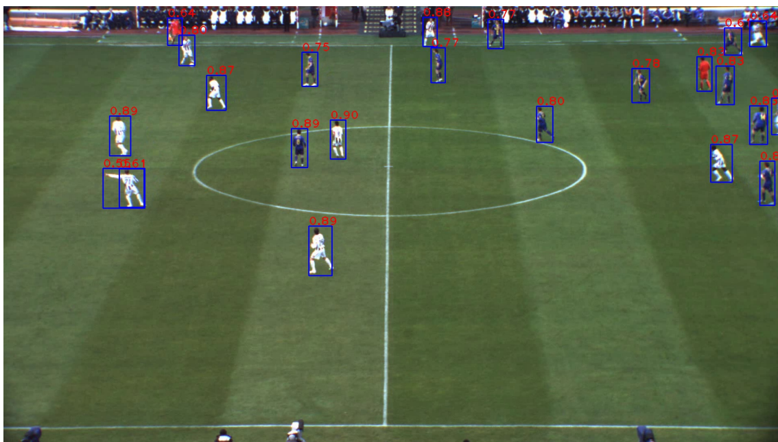
Figure 78: Examples of bad detections by the finetuned FairMOT model. The leftmost player is incorrectly labeled as two different objects. The smaller (incorrect) box has a large overlap with the correct one.
