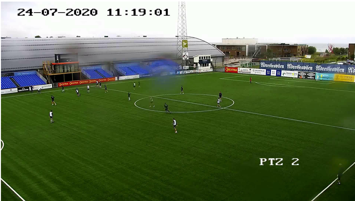
From the first video. Note how the overcast is influencing light conditions. Rain cause droplets to form on the lens.
