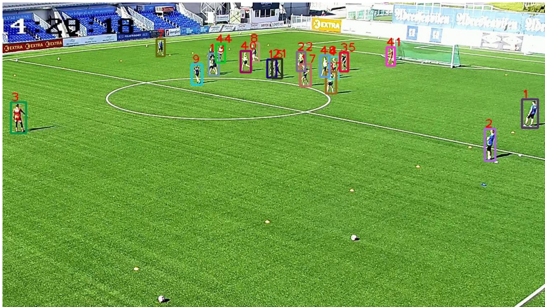
Figure 77: YOLOv5 + DeepSORT tracking demo on the Ranheim validation sequence. The sequence is very similar to data the model has trained on. The tracking is fragmented due to missed detections. A video demo can be viewed here , and here [101].
