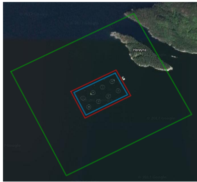
Figure I.1: The Green line show the outer geofence zone, the red line shows the inner geofence zone.
