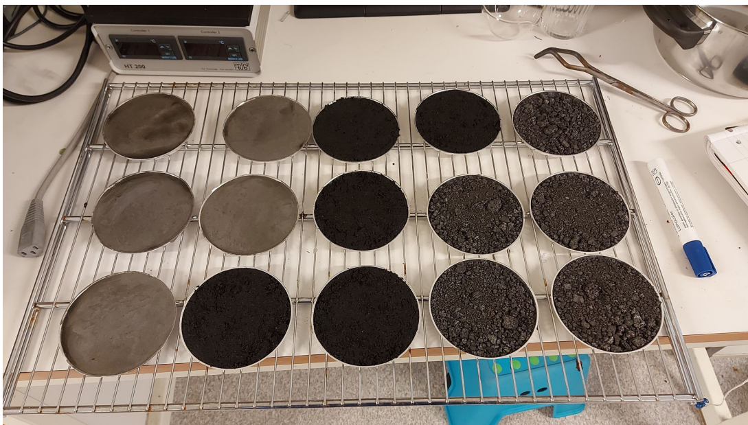
Figure 21: Tray of samples. On the left side, aluminium oxide. In the middle is anode mass. To the right is petroleum coke. This tray is from the first experiment where weight and water activity was measured at 15 minute intervals.
