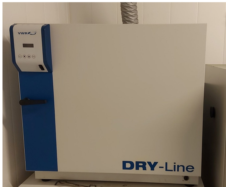
Figure 18: VWR DRY-Line Drying Oven DL53 with natural convection.
