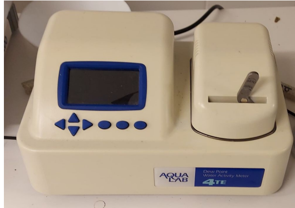
Figure 20: The water activity meter, AquaLab 4TE, was used in the experiments.
