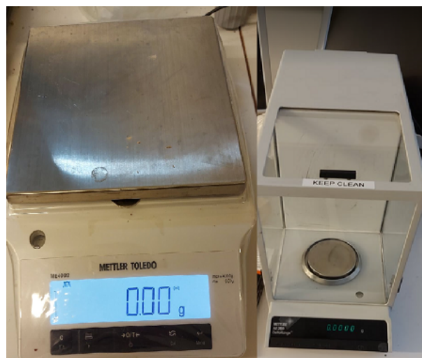
Figure 19: The weights: Mettler Toledo - Precision Balance ME4002 (left); and Mettler AE260 DeltaRange (right), were used in the experiments.
