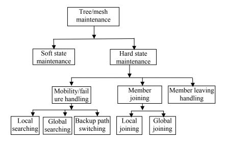
**Figure 3.** Classification of tree/mesh maintenance mechanisms.
