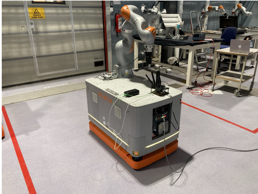
Figure 5.1: The setup at NTNU Gløshaugen’s Industry 4.0 laboratory. The 5G Raspberry Pi is powered by a portable charger and connected to a KMR iiwa entity with an Ethernet cable.
