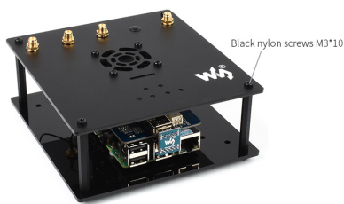
(g) Step 7: Assemble the top cover and fix with screws.
