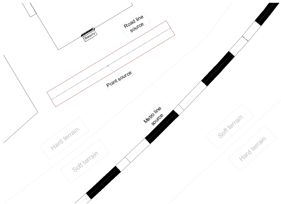
Figure 3.10: Birds eye view of position of balcony in relation to point source, road line source and metro line source in CadnaA simulation. The picture is purely illustrative, as the road source and metro source in the simulations are replaced with line sources, to make calculations based on the industry method of Nor96.
