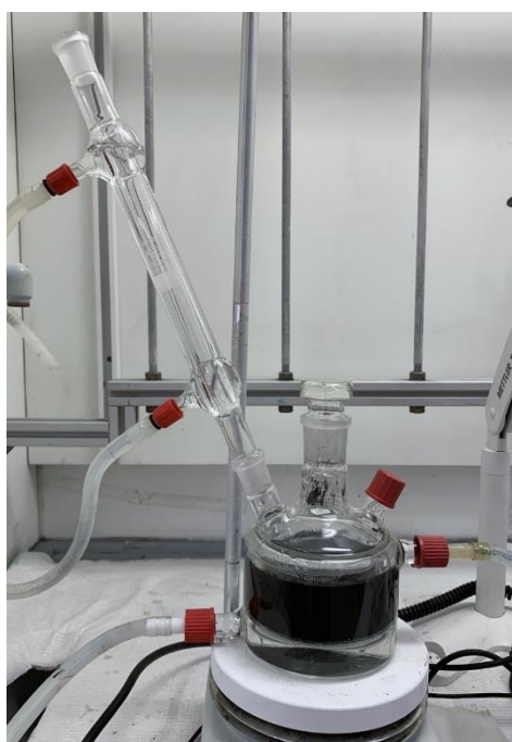
Figure 2.2. Leaching set-up. 250 mL glass reactor connected to heating circulator and condenser.
