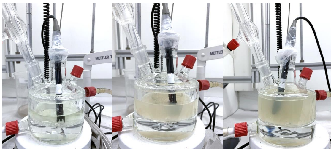
Figure 2.4. Precipitation of lithium carbonate by addition of \text{Na}_2\text{CO}_3 , showing (a) no addition, (b) directly after addition and (c) at the end of precipitation.
