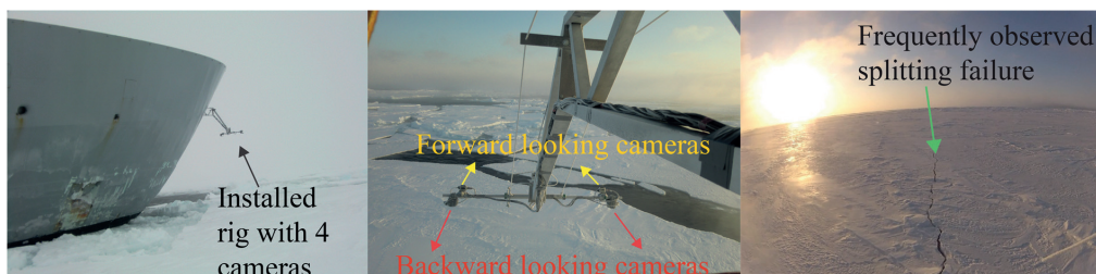
Fig. 2 Video camera system onboard KV Svalbard and frequently observed splitting failure of a large ice floe (March, 2012).
