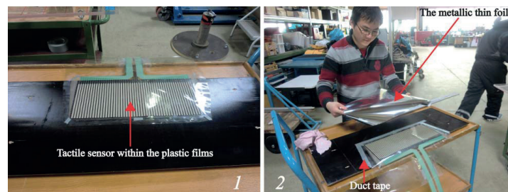
Figure 2 Installation of the tactile sensor on the sloping plate.
