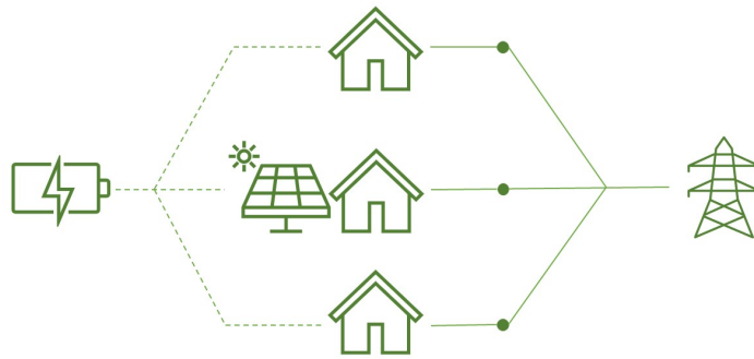
Figure 4.4: Illustration of configuration 4, where the buildings are metered individually and the battery capacity is shared within a local energy market.
