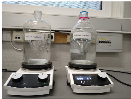
(a) Magnetic stirrers at RT were used to thoroughly mix and degass brines contained in the two containers shown
