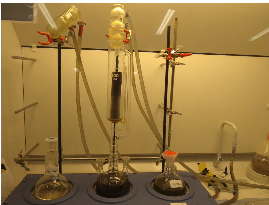
Figure 4.7: Core cleaning by Soxhlet. Methanol and Toluene were used as cleaning solvents
