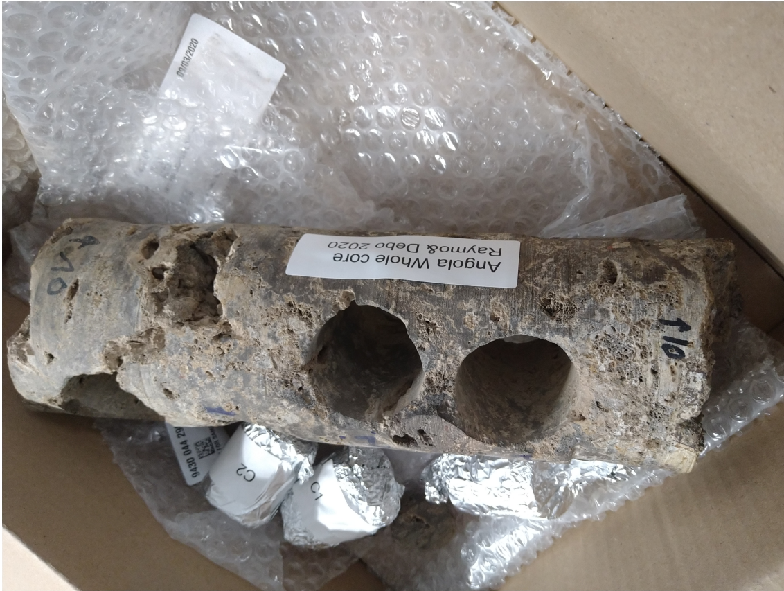
Figure 4.1: Angola Core plugs were dry drilled from this whole core in a direction parallel to the bedding. Deep vugs on the left of the core and the general rough texture hint on the extent of heterogeneity
