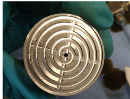
(b) Grooved end piece in contact with the core improved core-core holder end-piece contact
