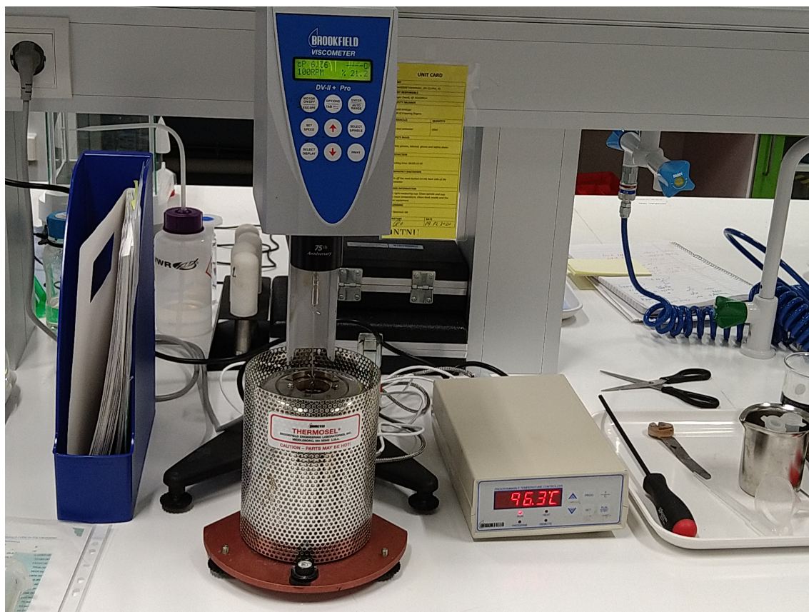
Figure 4.11: Viscosity measurements set up. The heating chamber, with red digits, made it possible to make measurements at 96°C
