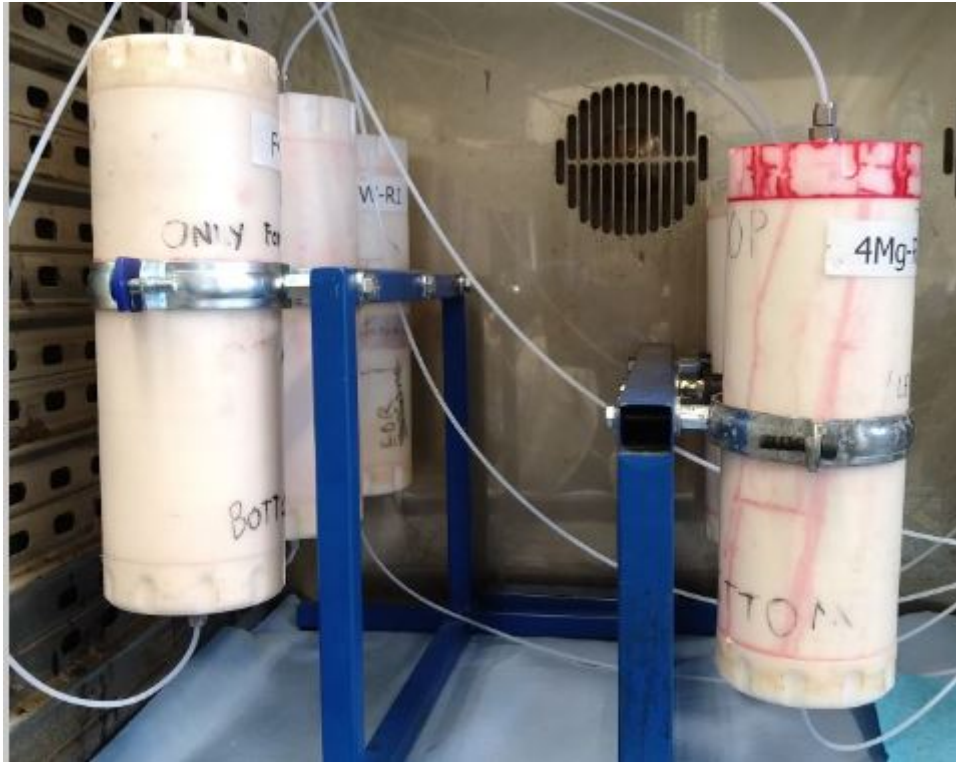
Figure 4.18: Brine reservoirs held in vertical position with steel stands. PTFE lines are connected to the reservoirs
