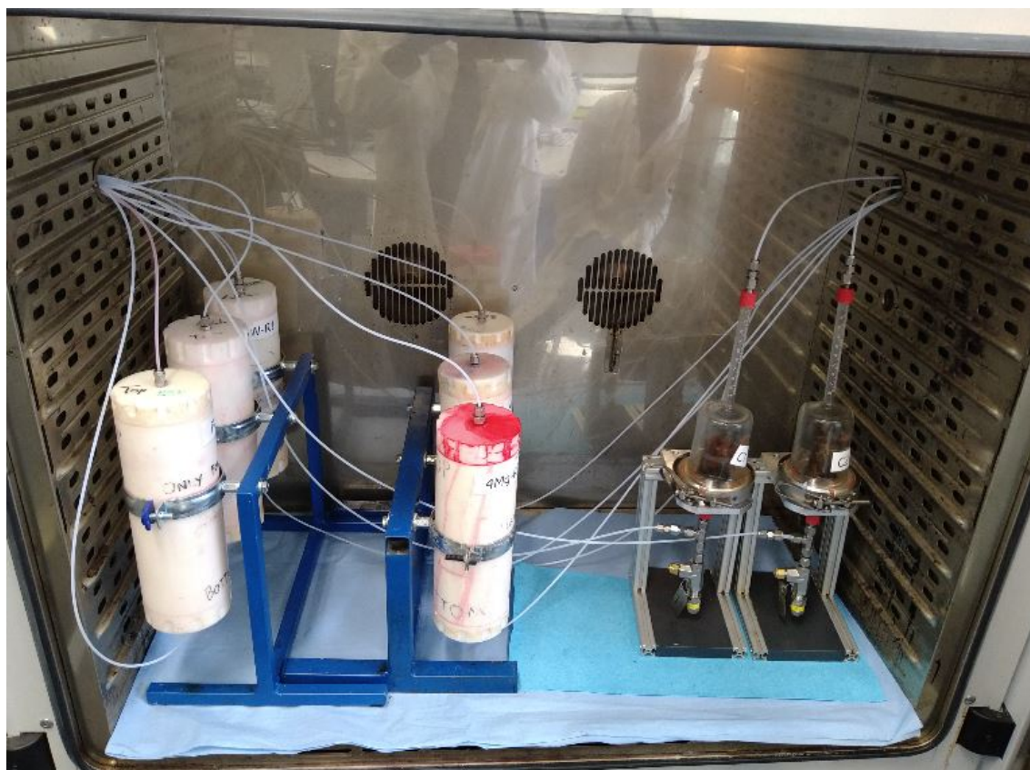
Figure 4.12: SI rig internal arrangement. The 6 white cylinders clamped on blue stands are the brine reservoirs. They are connected with white PTFE lines to the two Amott cells on the right. Not the pressure relief valves installed at the base of each Amott cell.
