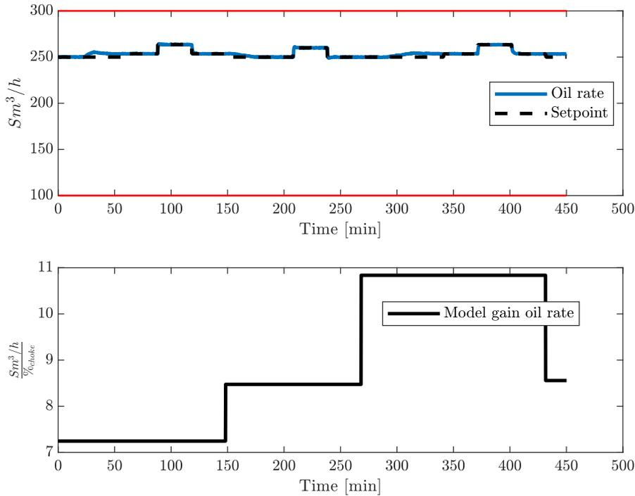
Figure 6.15: Process simulation of oil rate and the model gain updates, through disturbance changes. Oil rate setpoint excitation.
