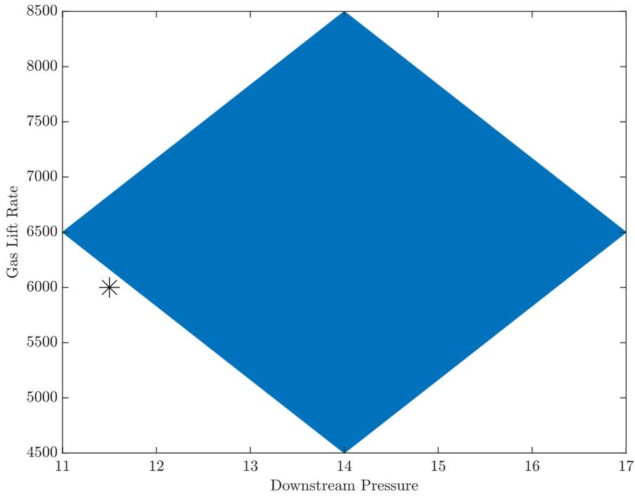
Figure 6.13: Initial acceptable area, with a gas lift rate of  $6500Sm^3/h$  and a downstream pressure of  $14bar$ . The asterisk shows where the disturbances are adjusted to after the initial model gains identification.
