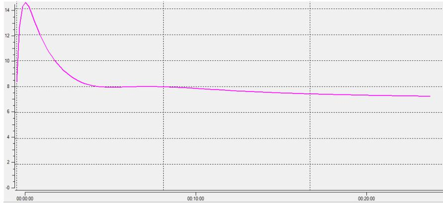
Figure B.1: Step response model, oil rate and choke. Steady-state gain:  $7.25 \frac{Sm^3/h}{\%choke}$ .
