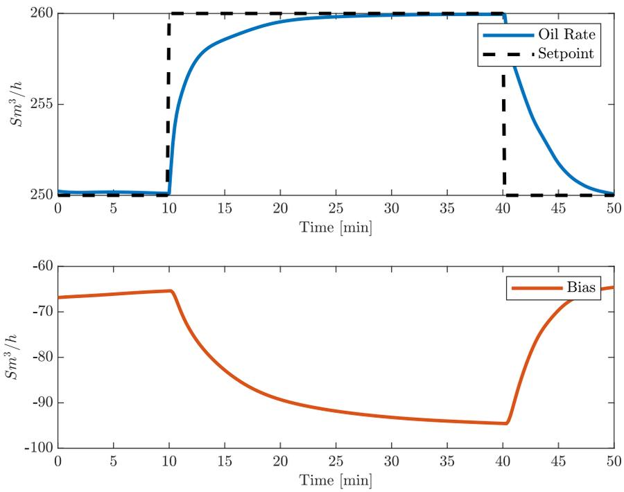
Figure 3.3: A process excitation with a poor mathematical model.
