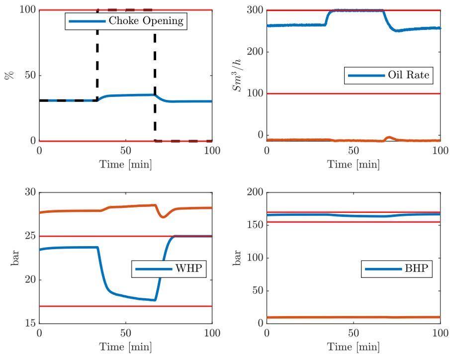
Figure 6.9: Ideal value procedure, with a gas lift rate of  $7500Sm^3/h$  and a downstream pressure of  $9bar$ , using the updated model gains. Model gains identified with production choke ideal value excitation, with a gas lift rate of  $7500Sm^3/h$  and a downstream pressure of  $9bar$ .
