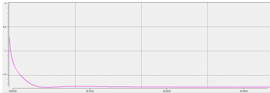
Figure B.2: Step response model, WHP and choke. Steady-state gain:  $-1.74 \frac{bar}{\%choke}$ .
