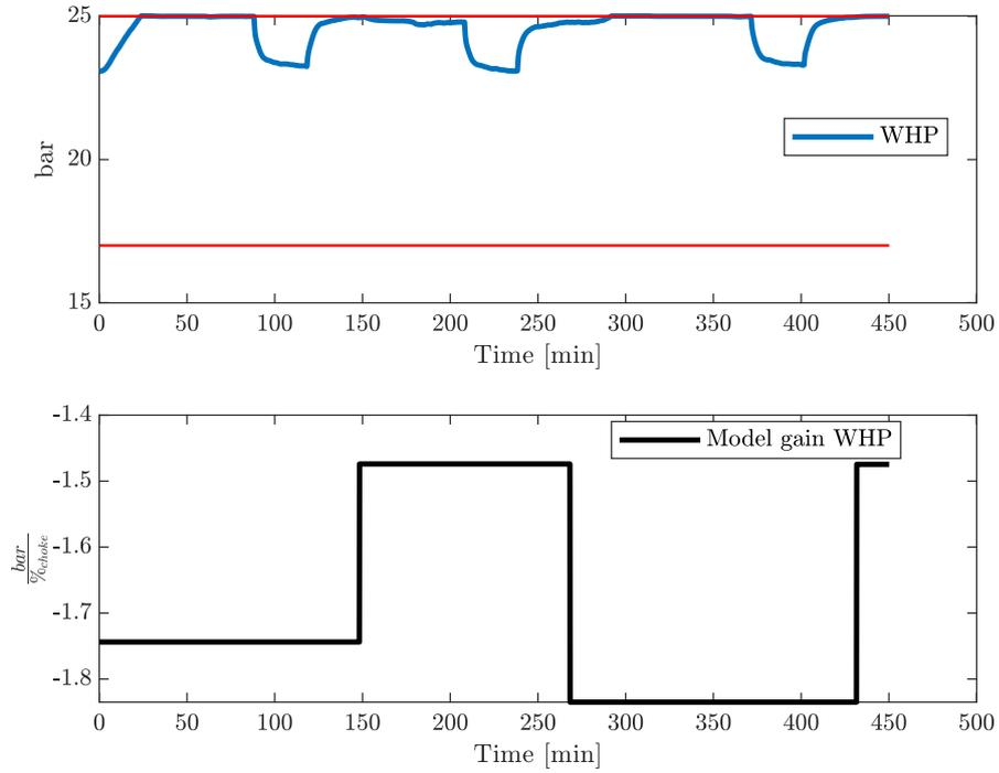
Figure 6.16: Process simulation of WHP and the model gain updates, through disturbance changes. Oil rate setpoint excitation.
