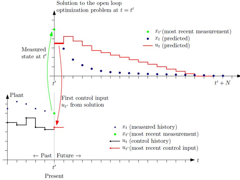
Figure 3.1: Illustration of the MPC principle [22].
