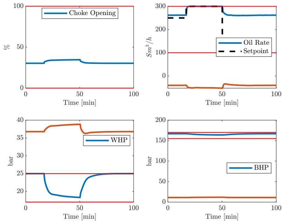
Figure 6.4: Setpoint procedure, with a gas lift rate of  $7500Sm^3/h$  and a downstream pressure of  $9bar$ , using the updated model gains. Model gains identified with oil rate setpoint excitation, with a gas lift rate of  $7500Sm^3/h$  and a downstream pressure of  $9bar$ .
