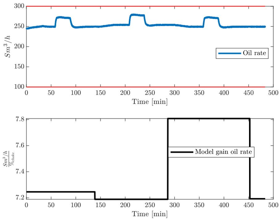
Figure 6.18: Process simulation of oil rate and the model gain updates, through disturbance changes. Production choke ideal value excitation.
