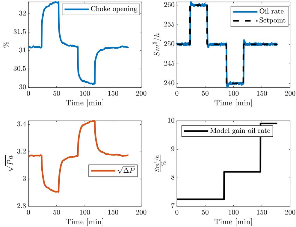
Figure 5.5: The process is first excited by moving the oil rate in positive direction, and then in negative direction. This yields two different model gains, respectively,  $8.2 \frac{Sm^3/h}{\%choke}$  and  $9.9 \frac{Sm^3/h}{\%choke}$ .
