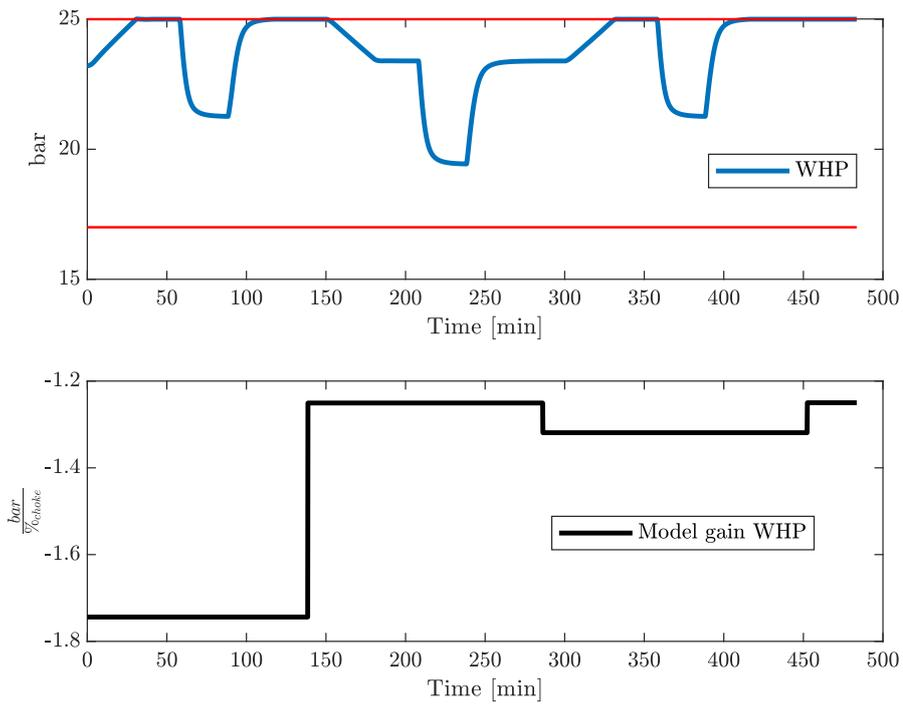
Figure 6.19: Process simulation of WHP and the model gain updates, through disturbance changes. Production choke ideal value excitation.
