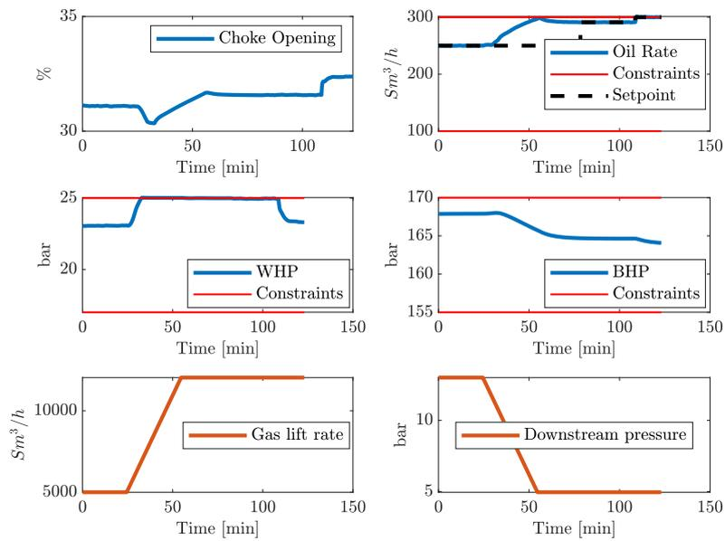
Figure 5.4: The disturbances changes and WHP reaches its upper limit. The automatic model gain identifier recognizes this, and the direction of the excitation step is positive as this is the direction which yields the maximum available excitation step. Excitation by moving the oil rate setpoint. The oil rate reaches its upper limit.
