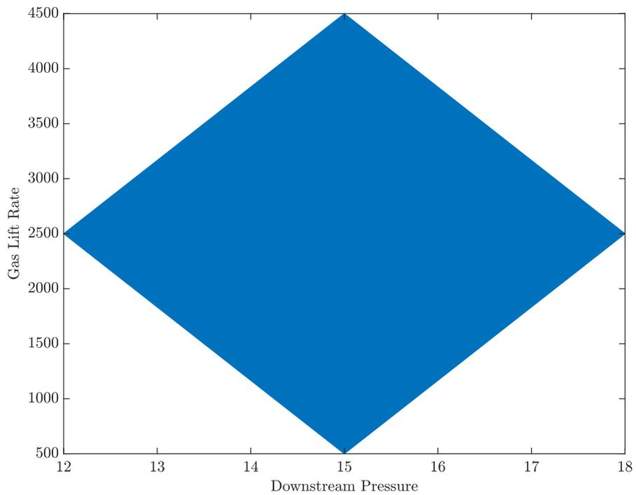
Figure 6.2: Updated acceptable area for the disturbances, after model gains identification at a gas lift rate of  $2500Sm^3/h$  and a downstream pressure of  $15bar$ .
