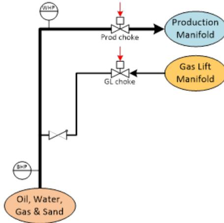
Figure 4.1: Simplified version of the subsea well system which the automatic model gain identifier is tested on [1].
