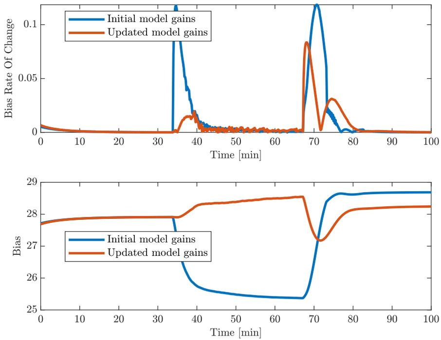
Figure 6.11: Comparing WHP absolute value of bias rate of change and bias between the initial and the updated model gains for the ideal value procedure.
