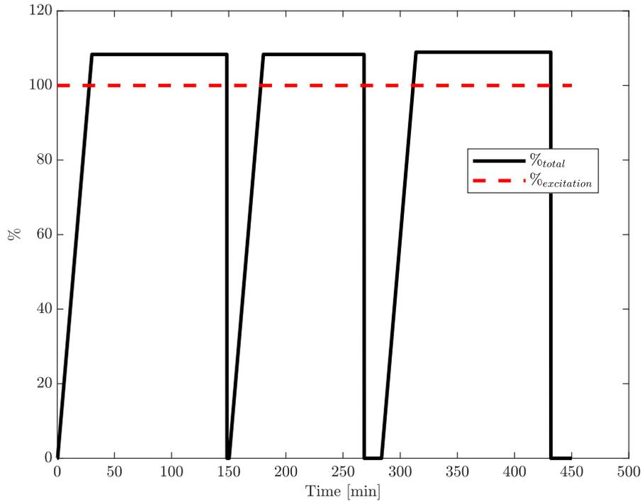
Figure 6.14:  $\%_{total}$  during the setpoint excitation simulation in Part 2.  $\%_{total}$  resets to 0 after implementing identified model gains.
