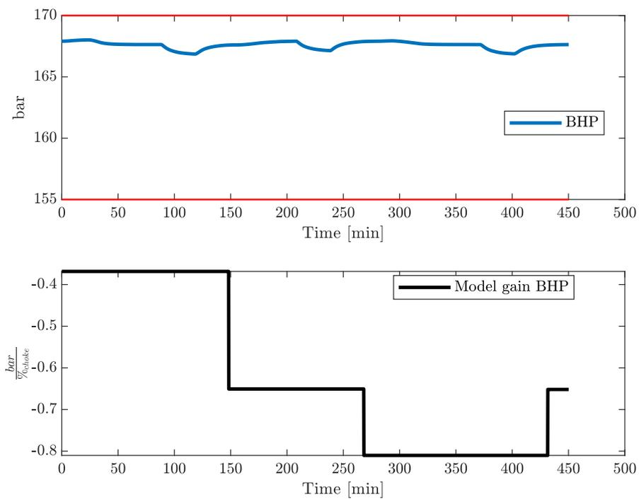
Figure 6.17: Process simulation of BHP and the model gain updates, through disturbance changes. Oil rate setpoint excitation.
