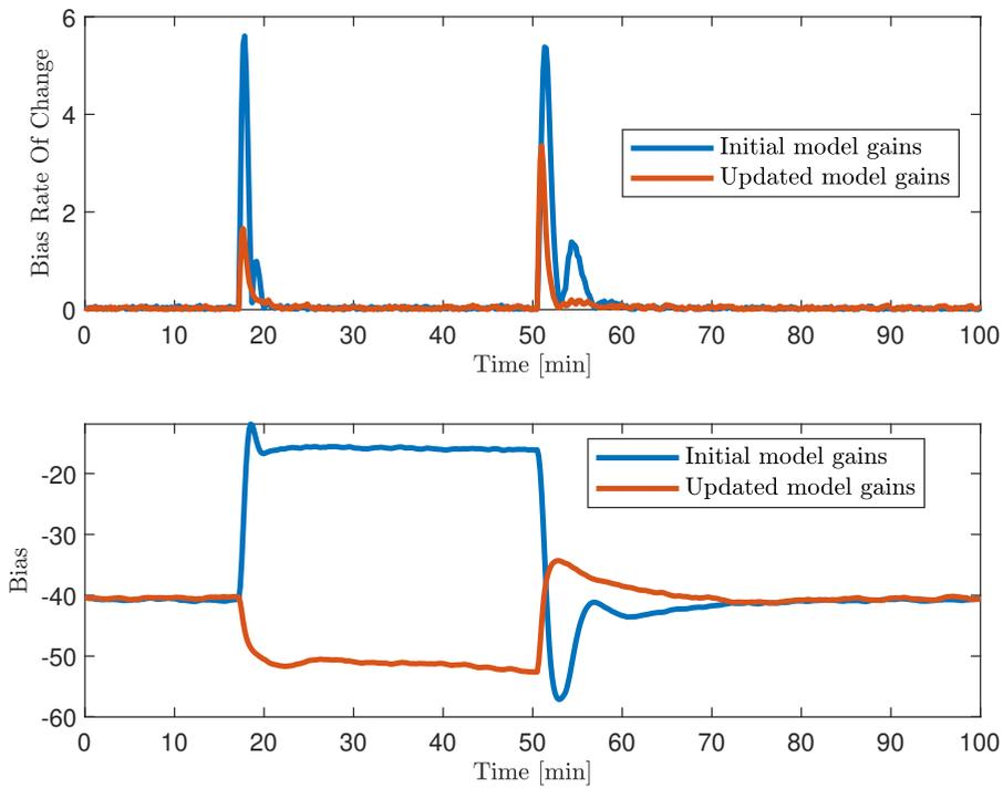
Figure 6.5: Comparing oil rate absolute value of bias rate of change and bias between the initial and the updated model gains for the oil rate setpoint procedure.
