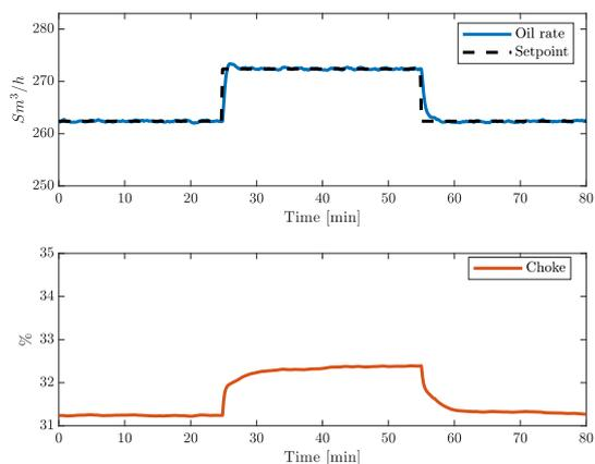
Figure 5.1: Excitation by moving the oil rate setpoint.
