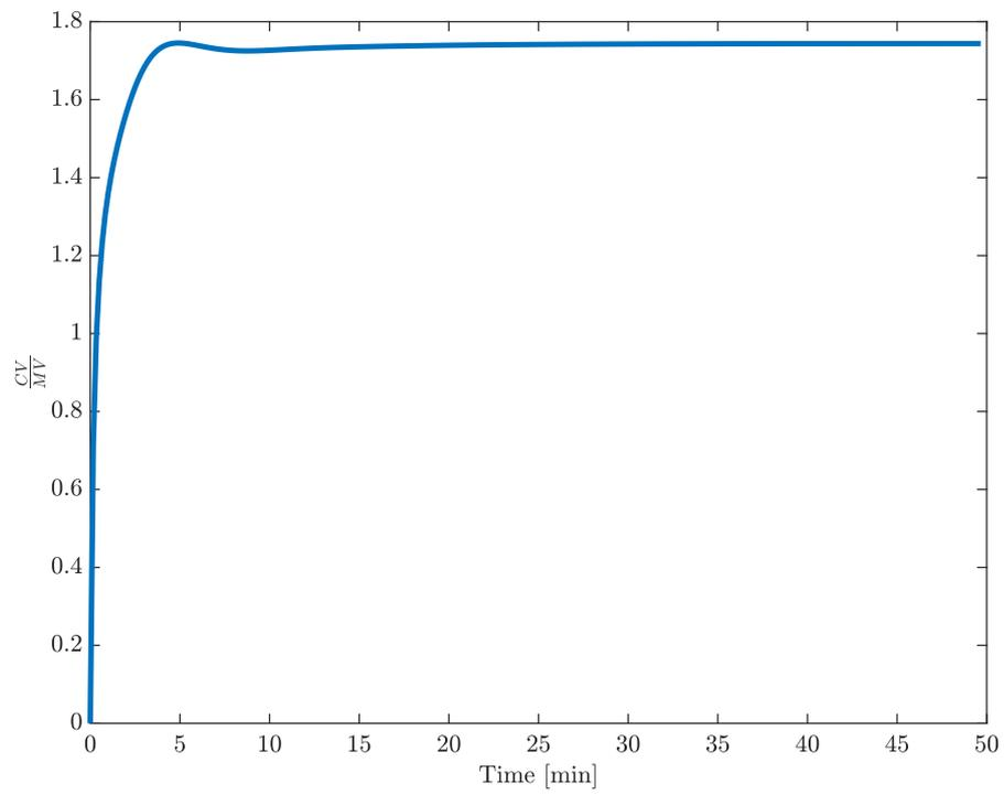
Figure 3.2: An example of a step response model in a SISO-system. A unit step in the MV yields the following response in the CV.
