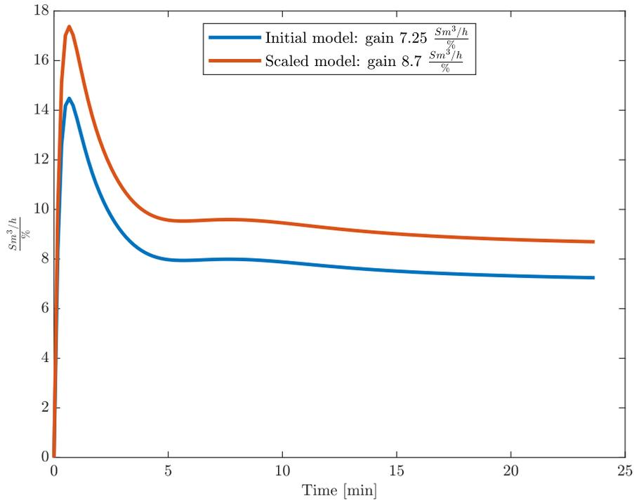
Figure 5.3: The initial step response model between oil rate and production choke, compared with the same step response model scaled by a factor of 1.2.
