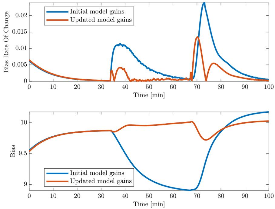
Figure 6.12: Comparing BHP absolute value of bias rate of change and bias between the initial and the updated model gains for the ideal value procedure.
