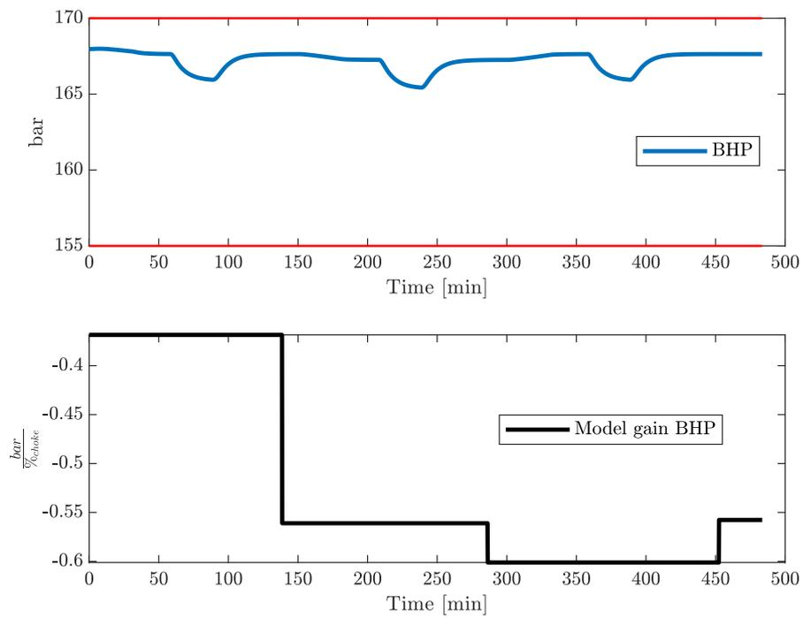
Figure 6.20: Process simulation of BHP and the model gain updates, through disturbance changes. Production choke ideal value excitation.
