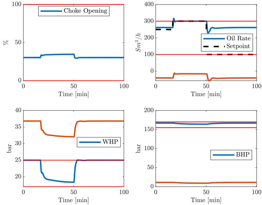
Figure 6.3: Setpoint procedure, with a gas lift rate of  $7500Sm^3/h$  and a downstream pressure of  $9bar$ , using the initial model gains. Model gains identified with oil rate setpoint excitation, with a gas lift rate of  $2500Sm^3/h$  and a downstream pressure of  $15bar$ .
