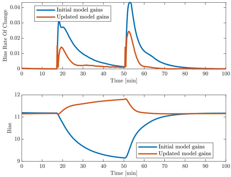
Figure 6.7: Comparing BHP absolute value of bias rate of change and bias between the initial and the updated model gains for the oil rate setpoint procedure.
