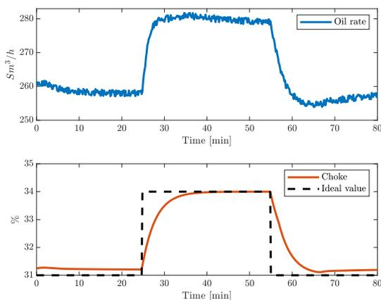
Figure 5.2: Excitation by moving the production choke ideal value.
