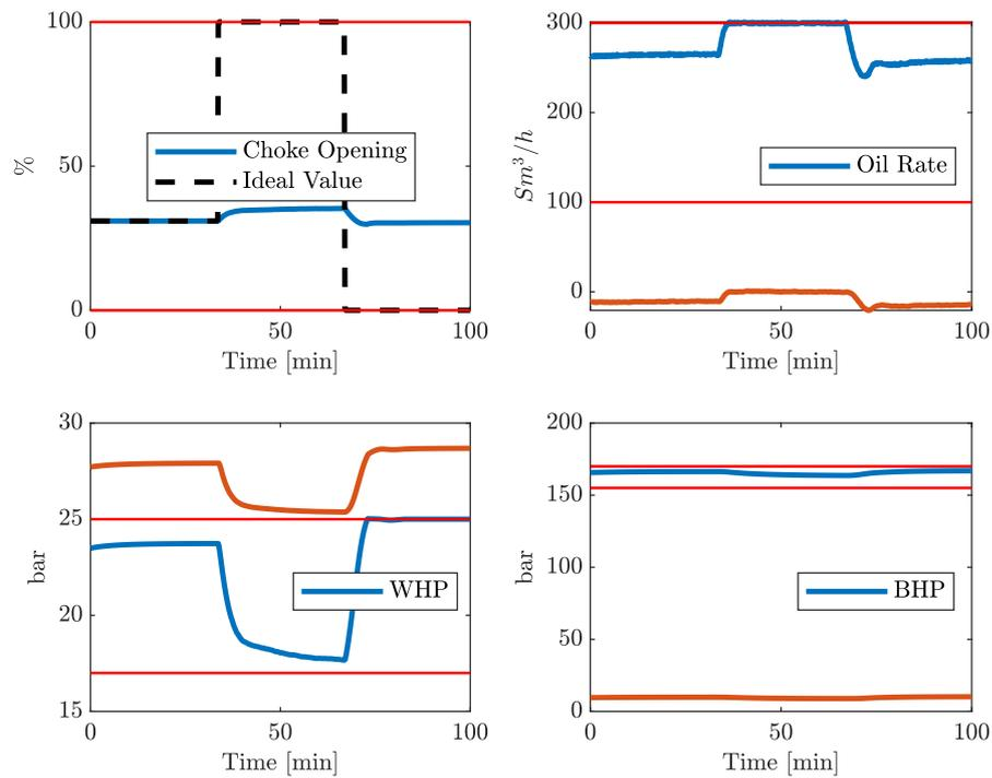
Figure 6.8: Ideal value procedure, with a gas lift rate of  $7500Sm^3/h$  and a downstream pressure of  $9bar$ , using the initial model gains. Model gains identified with production choke ideal excitation, with a gas lift rate of  $2500Sm^3/h$  and a downstream pressure of  $15bar$ .
