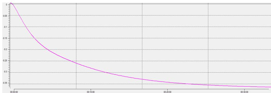
Figure B.3: Step response model, BHP and choke. Steady-state gain:  $-0.369 \frac{bar}{\%choke}$ .
