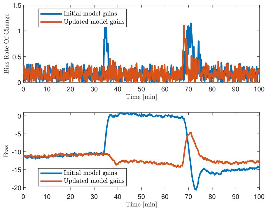
Figure 6.10: Comparing oil rate absolute value of bias rate of change and bias between the initial and the updated model gains for the ideal value procedure.
