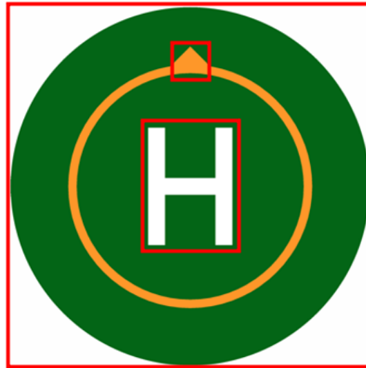
FIGURE 4.2: The landing platform with bounding boxes encapsulating the three classes; Helipad , H and Arrow .
