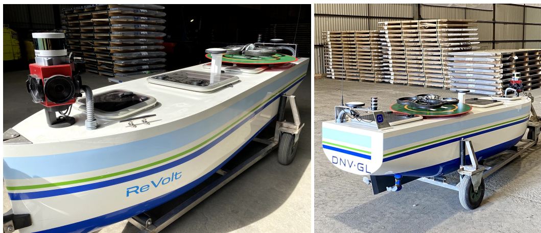
FIGURE 5.11: The DNV ReVolt with the landing platform mounted on the deck
