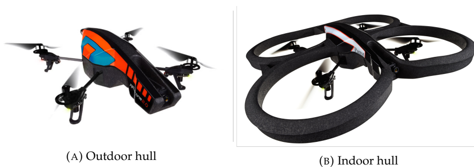
FIGURE 3.1: The Parrot Ar.Drone 2.0 with outdoor- and indoor hulls.
