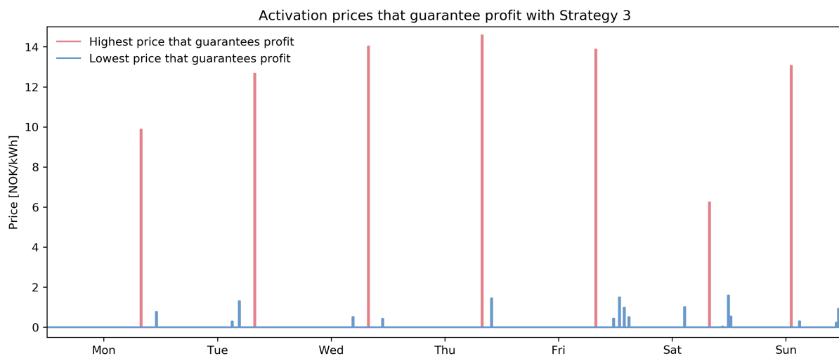
Figure 26: Feasible price range for ensuring profit for all participants for week 1, for Strategy 3 assuming uniform prices constrained between 0 and 100 NOK/kWh in every quarter of the day.
