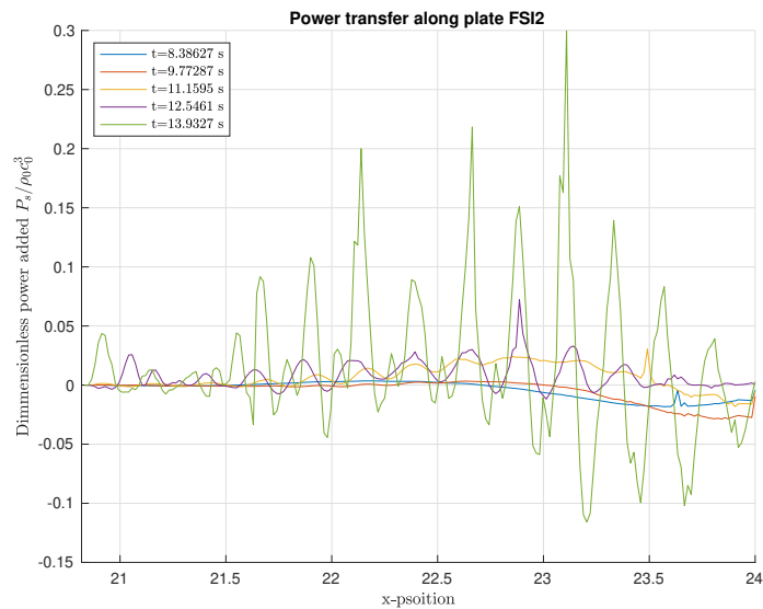
Figure 42: Non dimensional power transfer P_s = -\delta p \dot{\phi} / (\rho_s c_0^3) along tail at selected times for the FSI2 setup using the present 2nd order SBP method. A non dimensional time step of dt' = 3 \cdot 10^{-3} is used, and the second order low-pass filter is applied every 8th time step.
