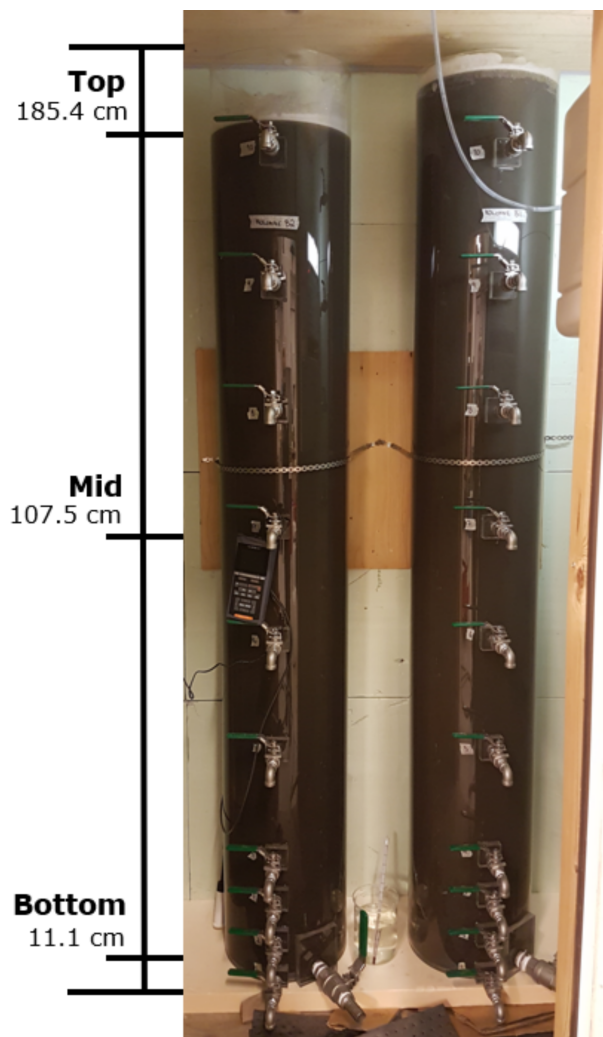
Figure 4: Sedimentation pilot setup consisting of two parallel columns with 2m height and 0.3 m diameter. The top, mid and bottom taps for extracting subsamples at discrete heights are indicated, with height measures from the interior bottom of the sedimentation pilot to the center of the taps. Illustrative water level difference between the two parallel columns.
