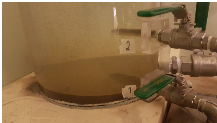
Figure 21: Sediment layer in the bottom of sedimentation column after 30 days of sedimentation, interfering with the lowermost extraction tap, marked "1" in the photo.
